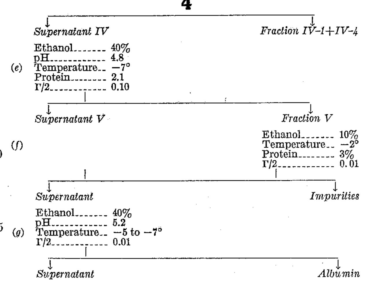
(a) 750 1. plasma is adjusted to pH 7.2 by addition of 2.6 1. sodium acetate-acetic acid buffer. The mixture is then brought to 8% ethanol concentration by addition of 132.8 1. 53.3% ethanol, while maintaining the temperature at  $-2.5^{\circ}$  (the time of ethanol addition being two hours). The precipitate (Fraction I) is removed by centrifugation at the rate of about 60 liters per machine per hour at  $-2^{\circ}$ .
