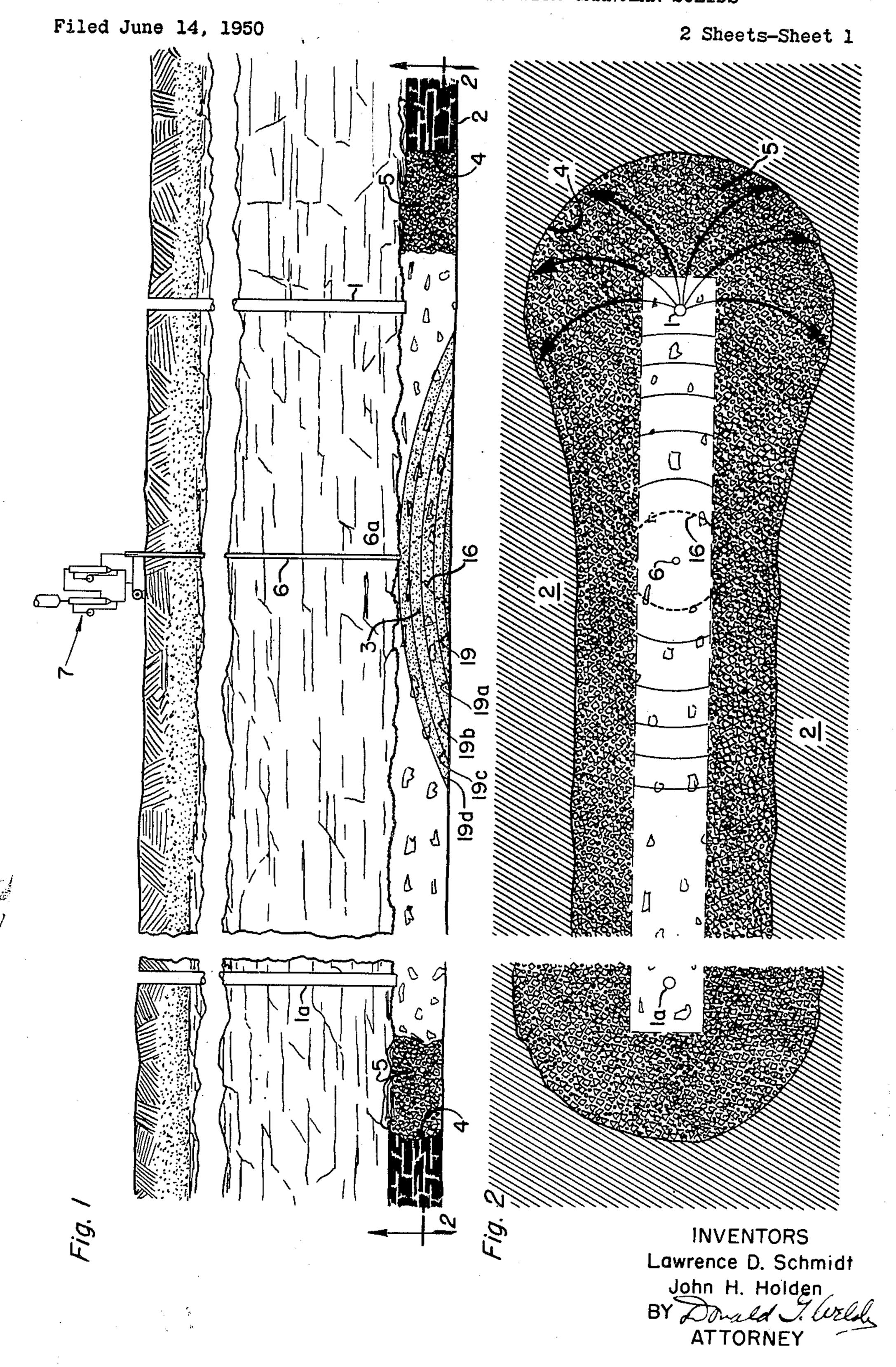
METHOD FOR FILLING CAVITIES WITH GRANULAR SOLIDS
