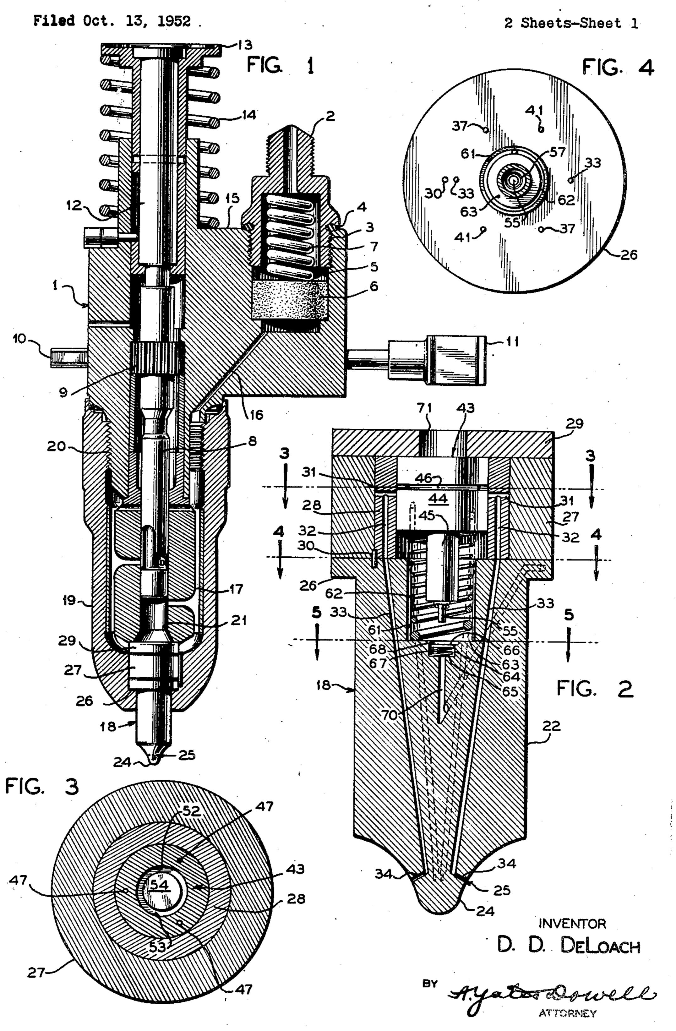
FUEL INJECTION APPARATUS FOR INTERNAL COMBUSTION ENGINES
