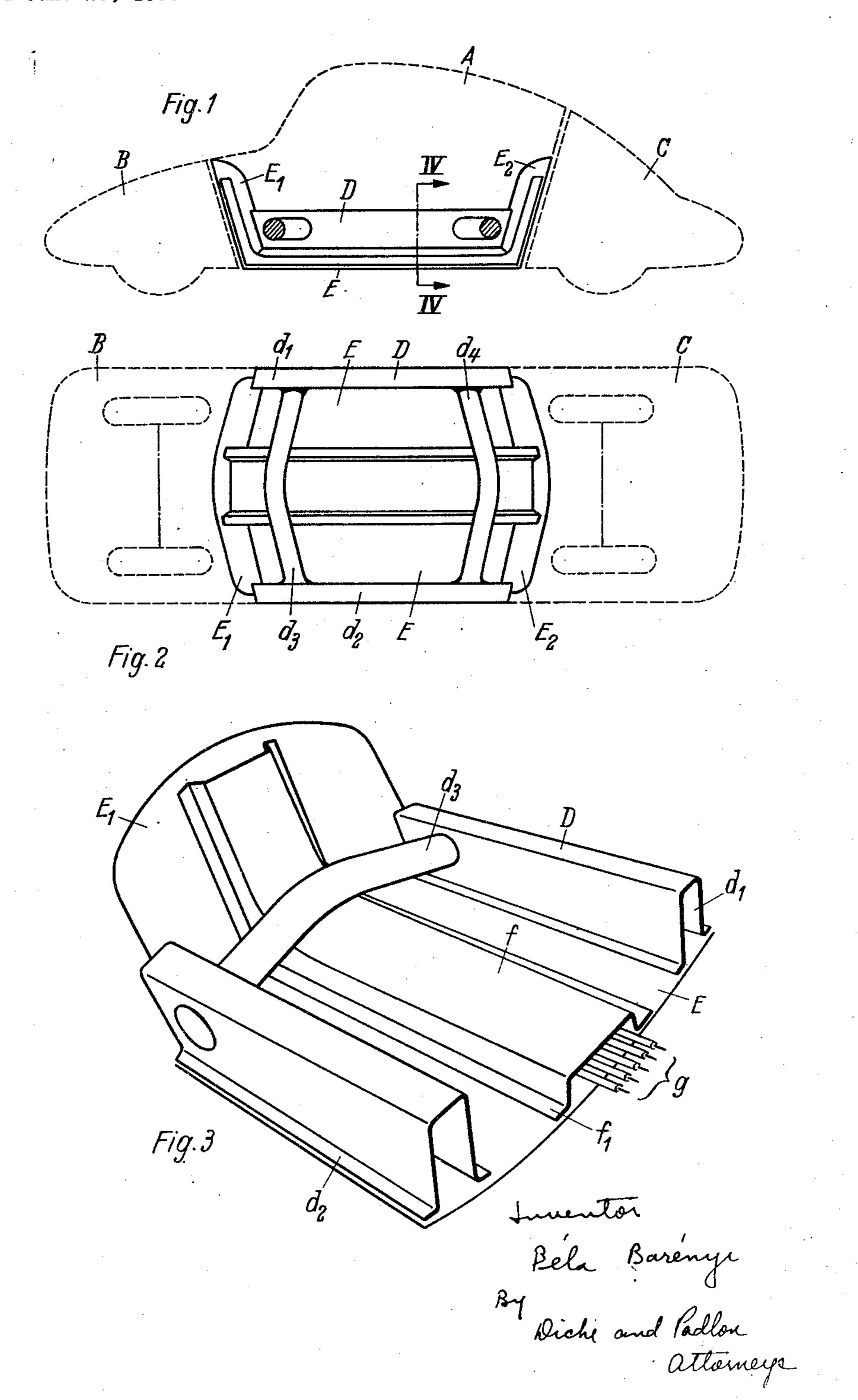
REINFORCED FLOOR PLATE FOR BODY OF SECTIONAL AUTOMOBILE
