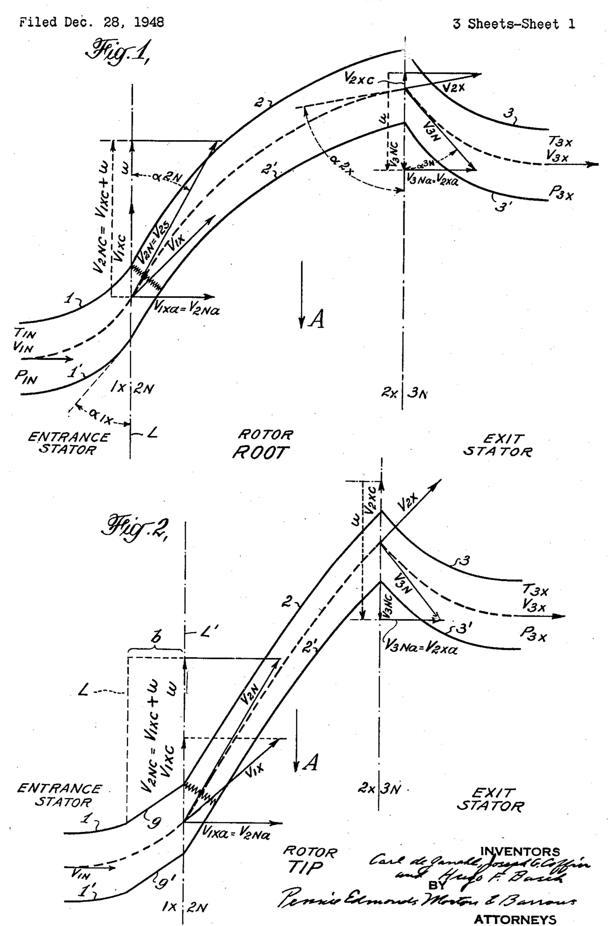
AXIAL FLOW COMPRESSOR Filed Dec. 28, 1948 3 Sheets-Sheet 2 AXIAL FLOW COMPRESSOR
