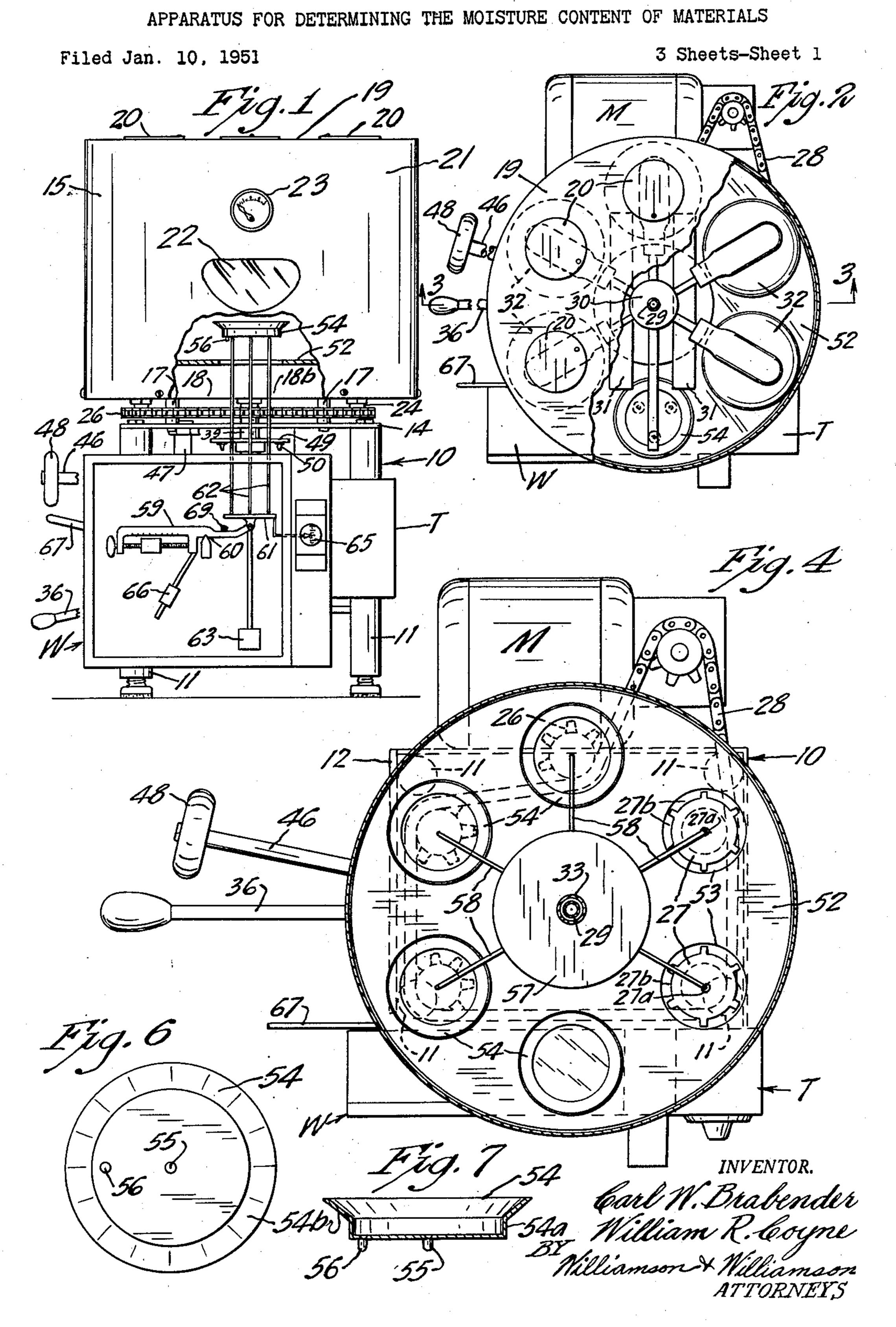
APPARATUS FOR DETERMINING THE MOISTURE CONTENT OF MATERIALS
