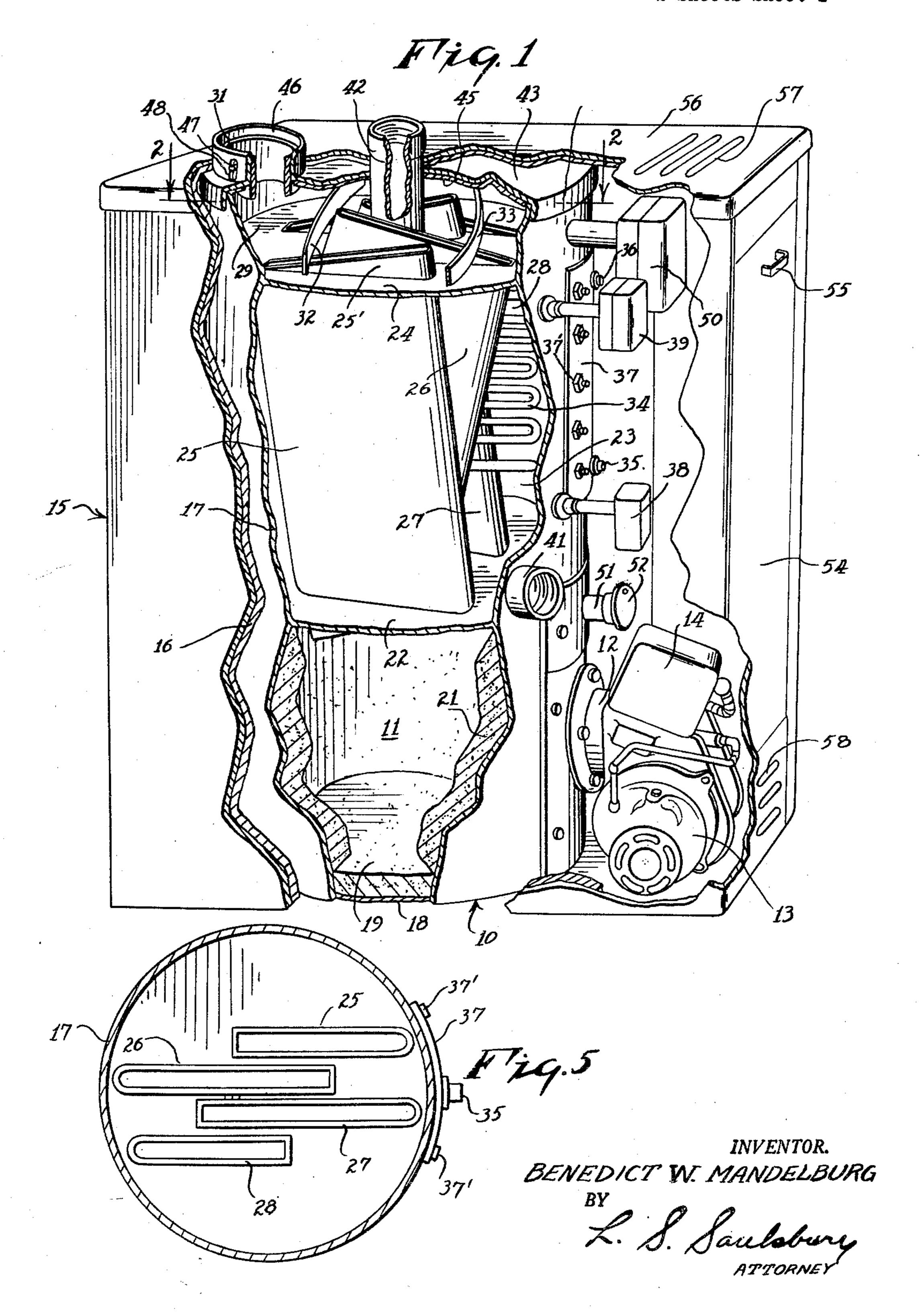
CROSSED DUCT VERTICAL BOILER CONSTRUCTION
