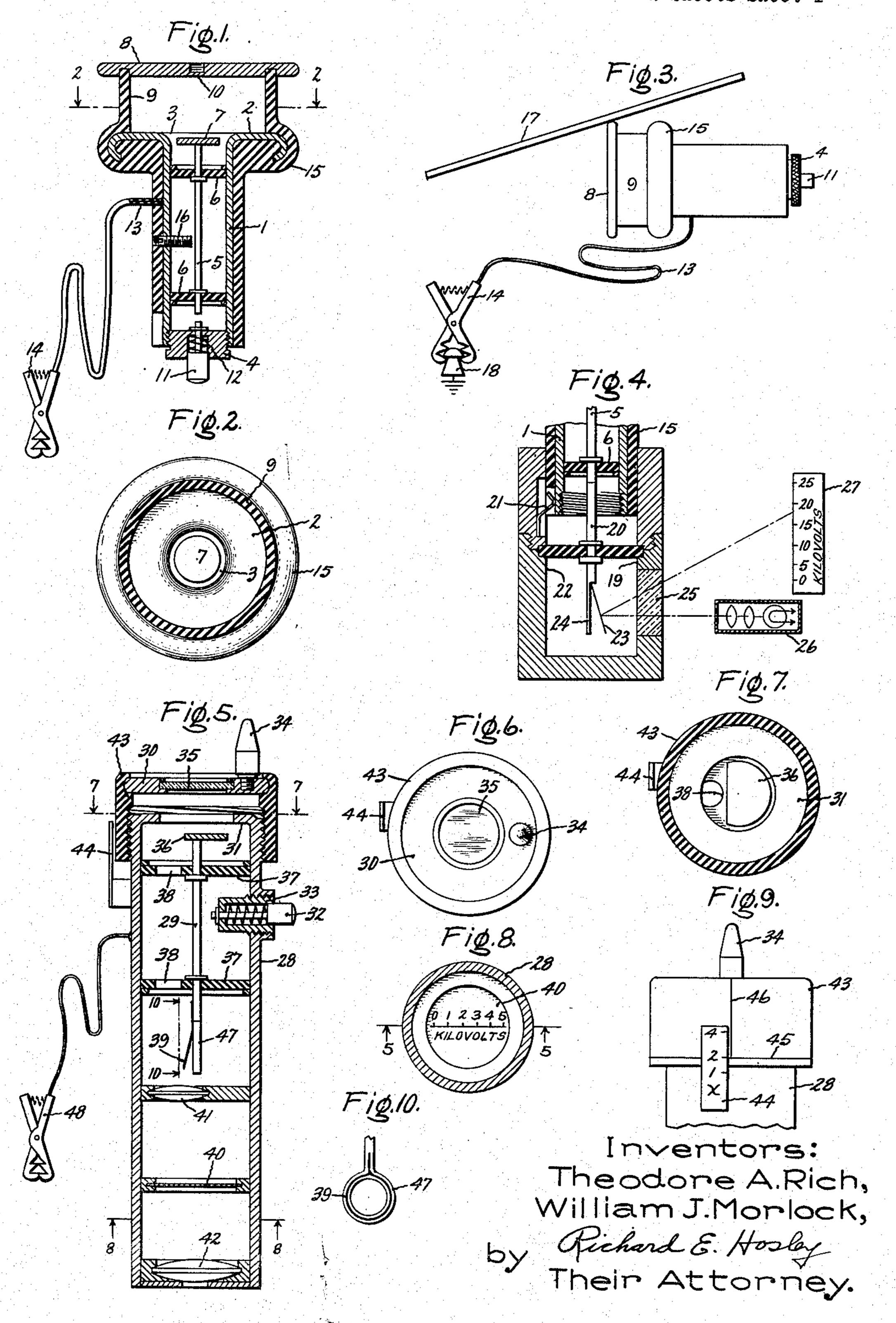
ELECTROSTATIC INDUCTION VOLTAGE MEASURING DEVICE
