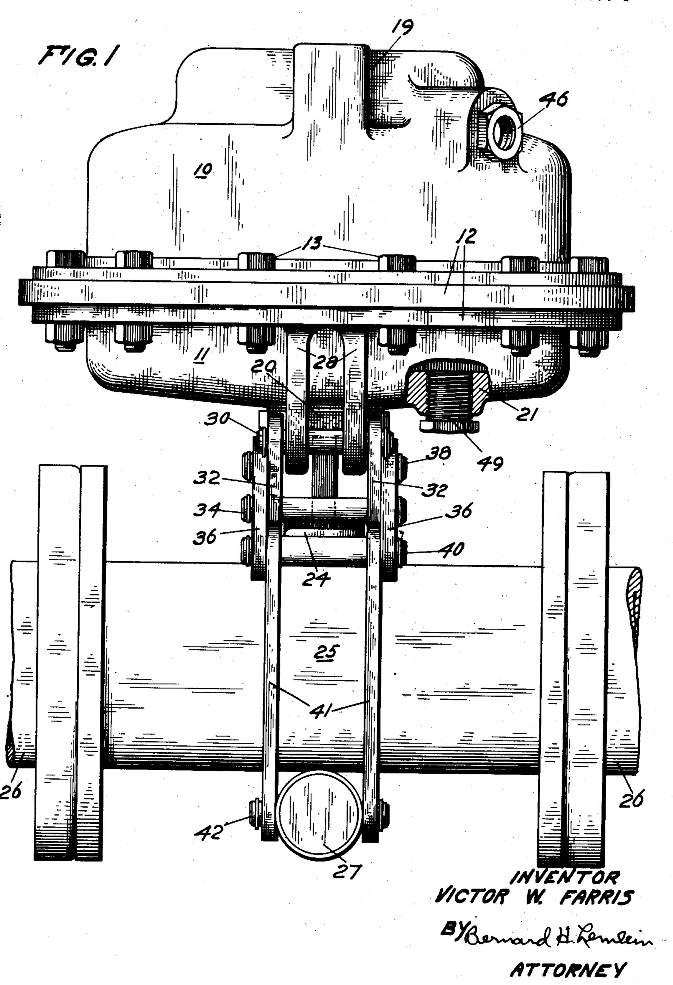
PINCH VALVE MECHANISM
