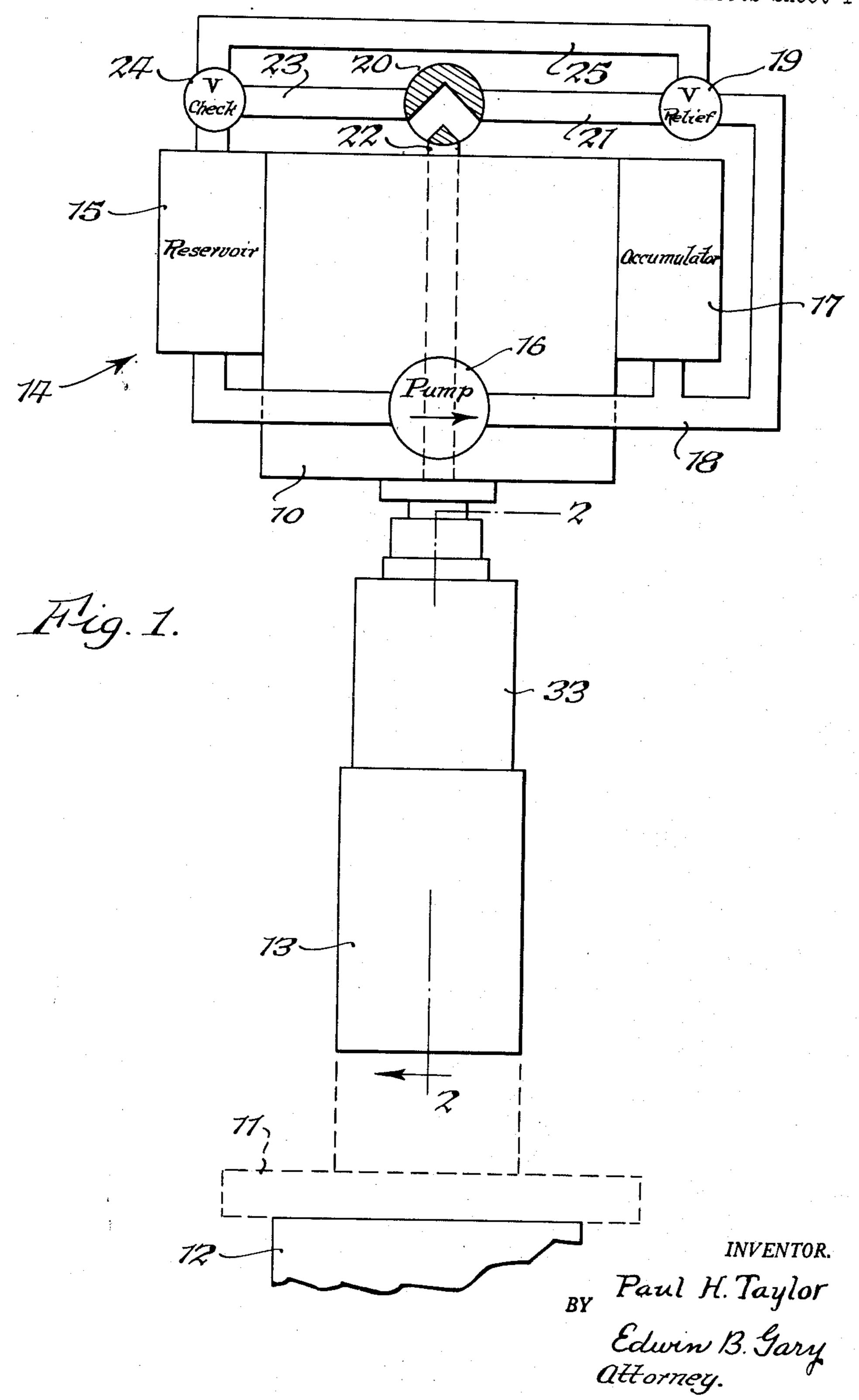
MACHINE TOOL WITH LIQUID-SPRING ACTUATED RAM
