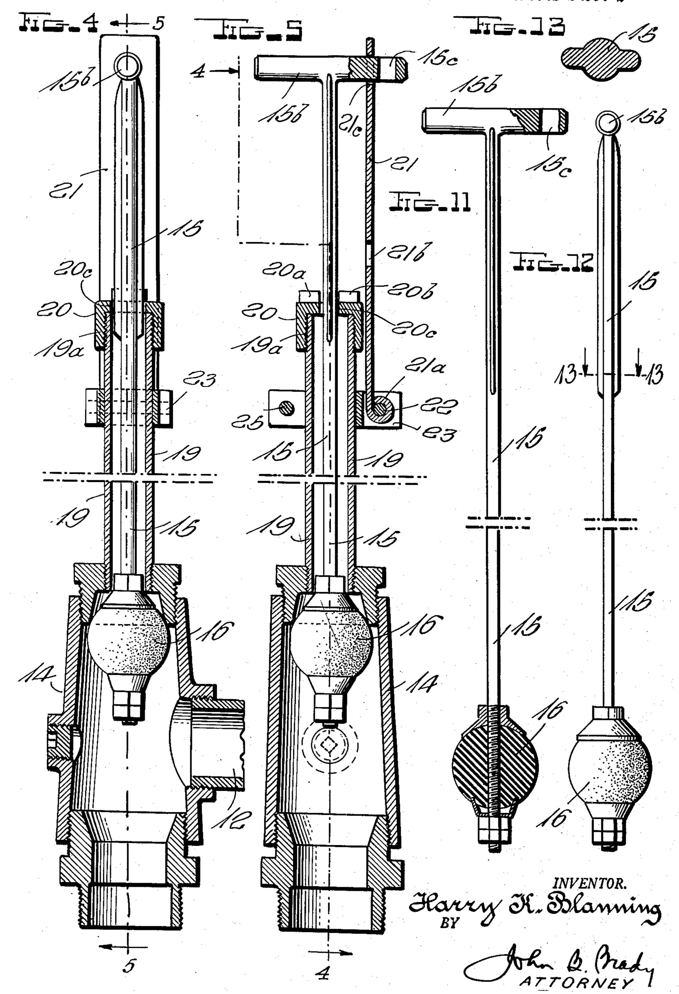
SEAL FOR VALVE ACTUATORS
