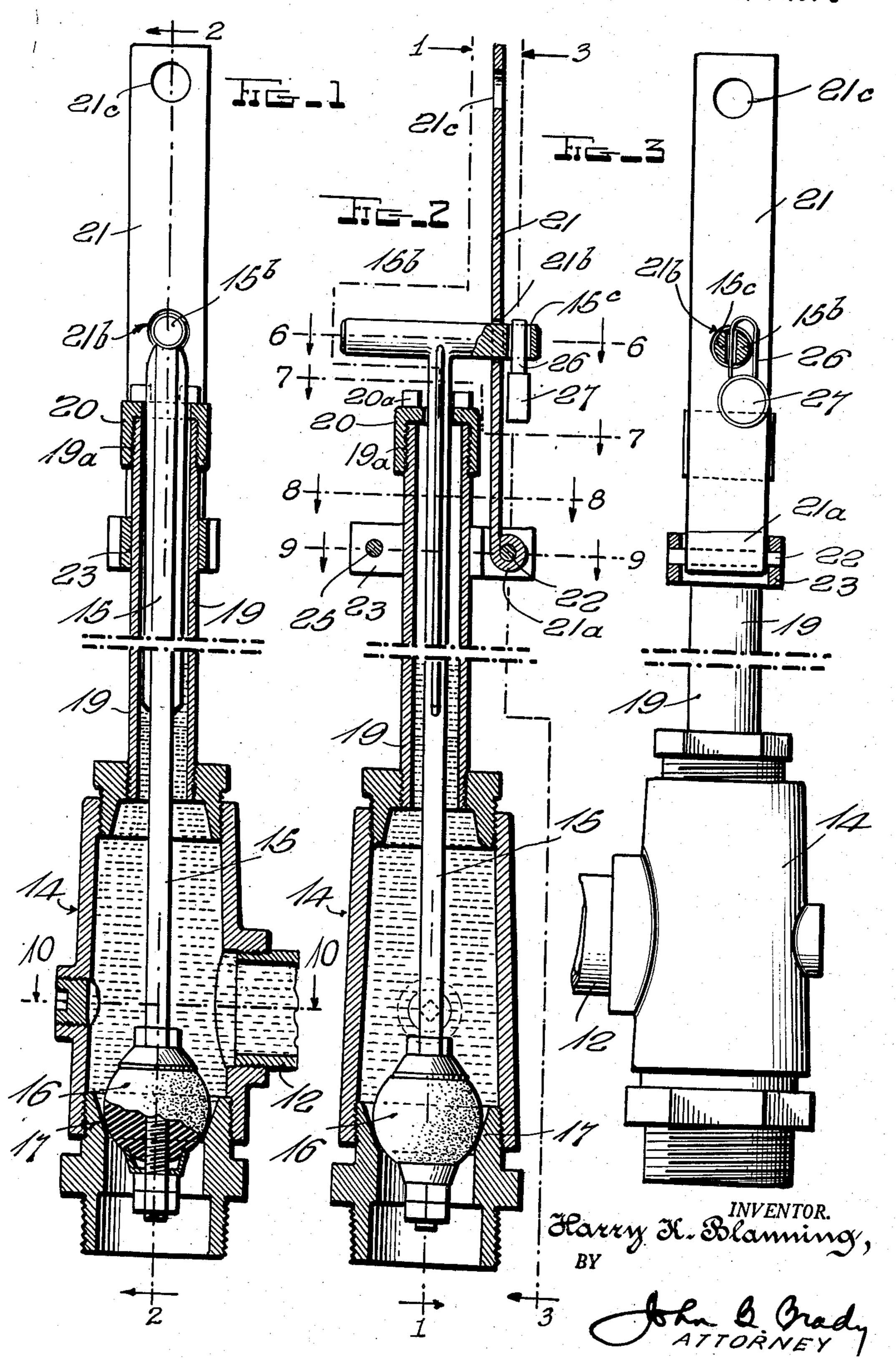
SEAL FOR VALVE ACTUATORS
