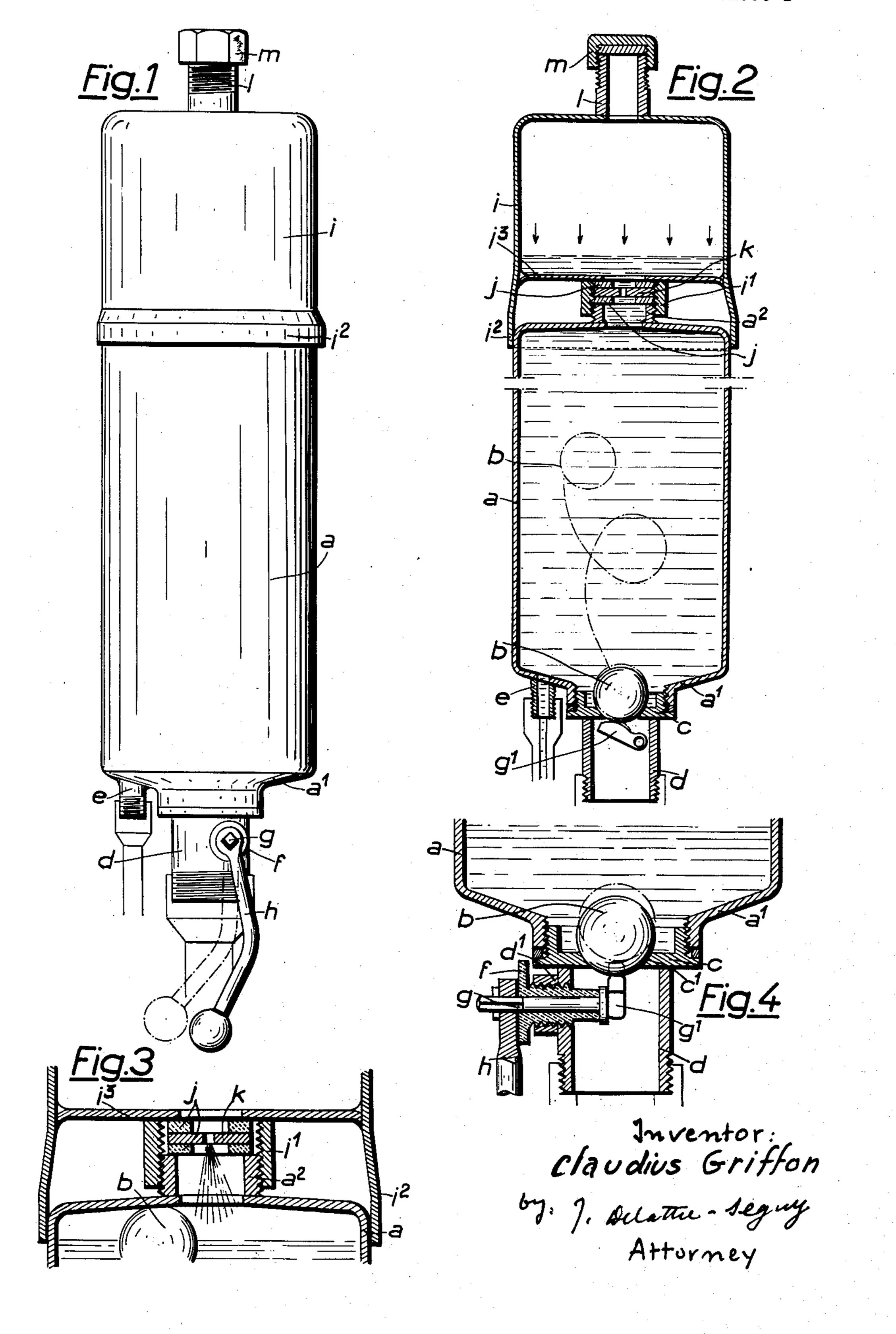
FLUSHING DEVICE FOR WATER CLOSETS
