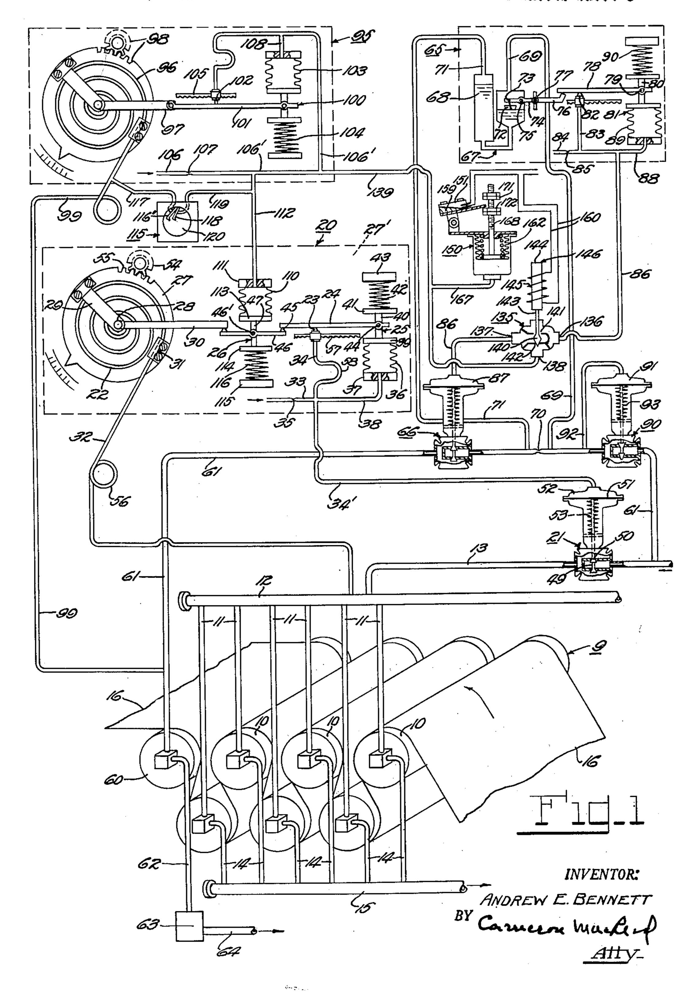
SHEET MOISTURE DRYING MACHINE CONTROL MECHANISM
