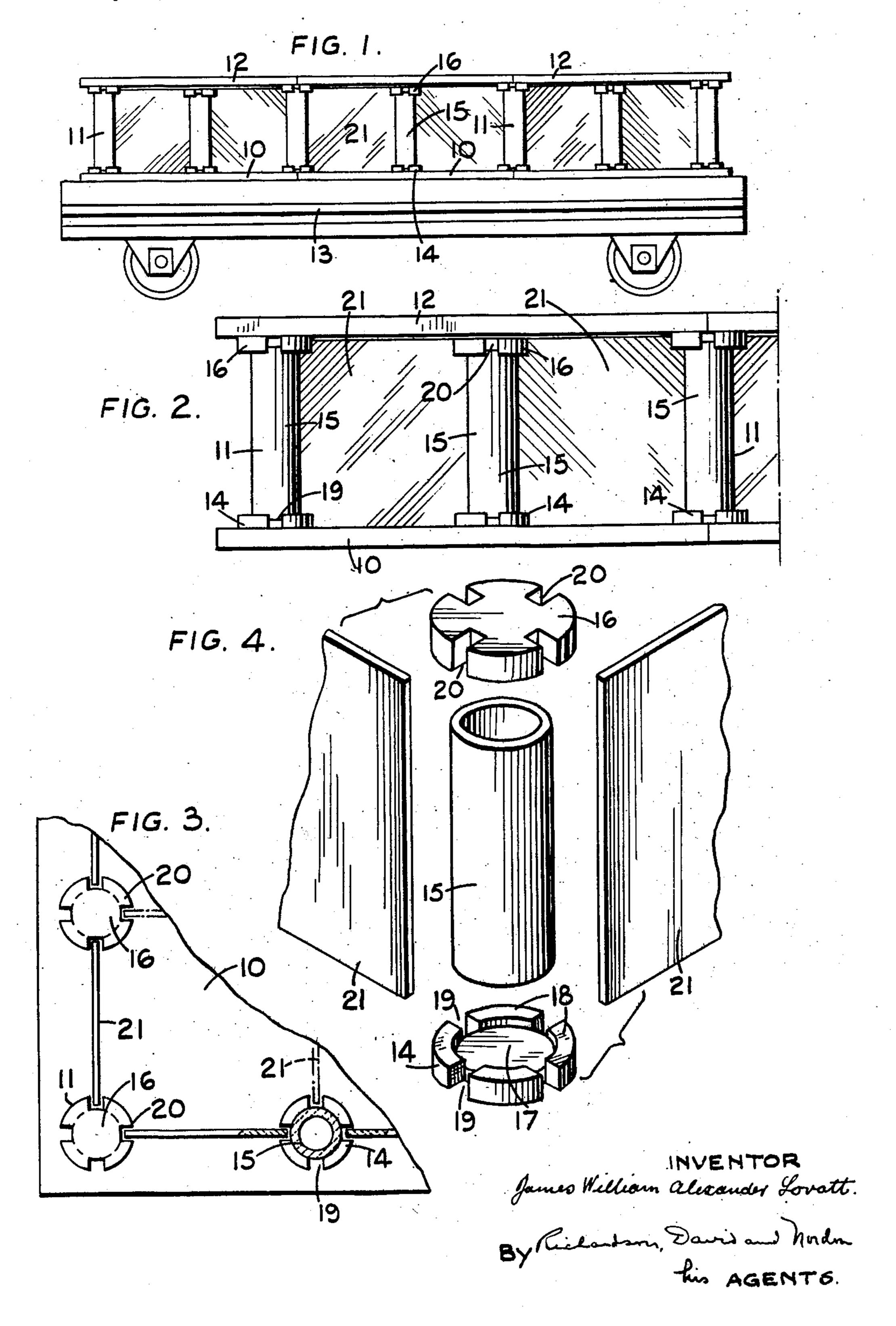
MUFFLE STRUCTURE FOR USE IN FIRING KILNS AND OVENS
