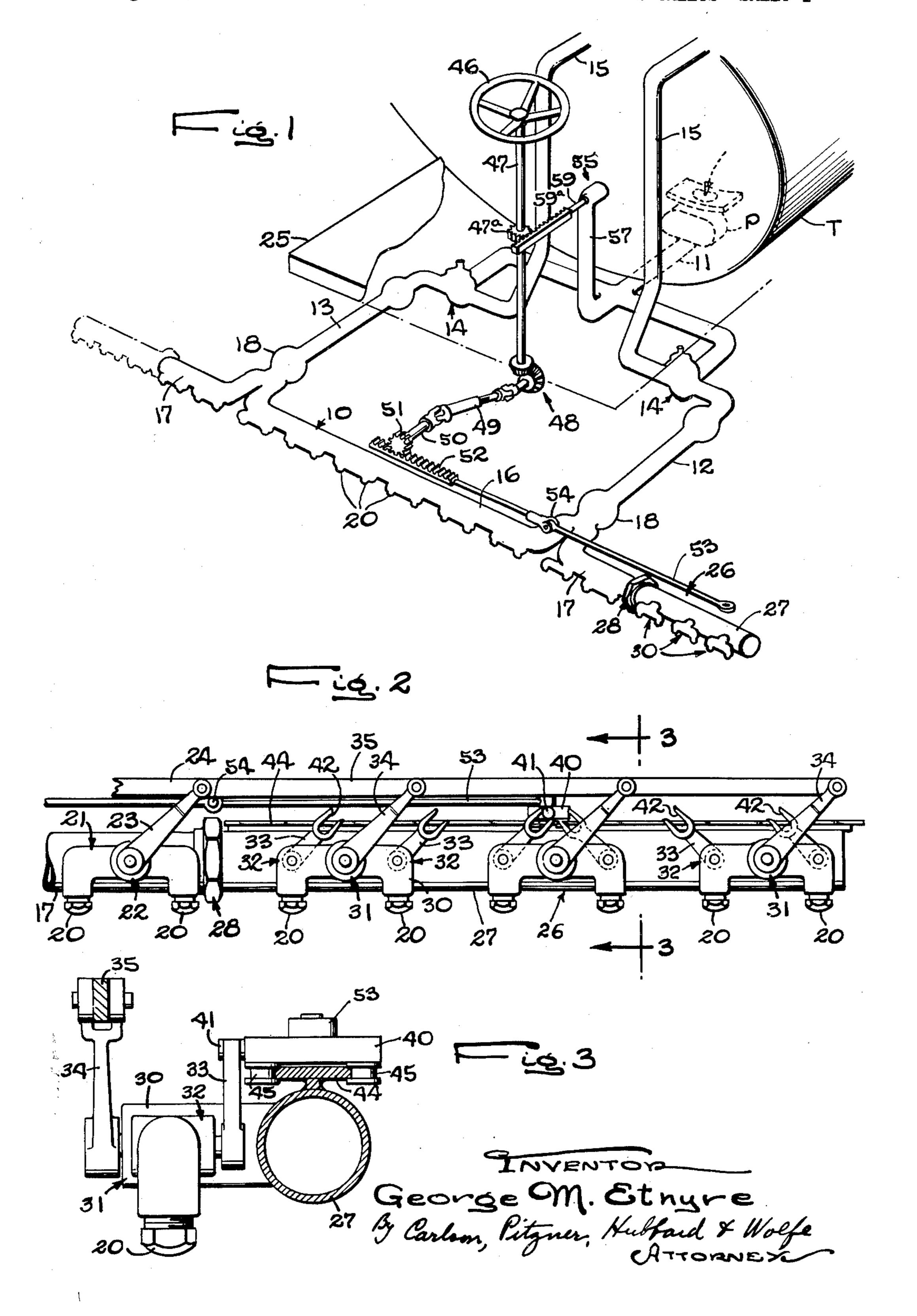
DISTRIBUTOR FOR BITUMINOUS AND LIKE MATERIAL
