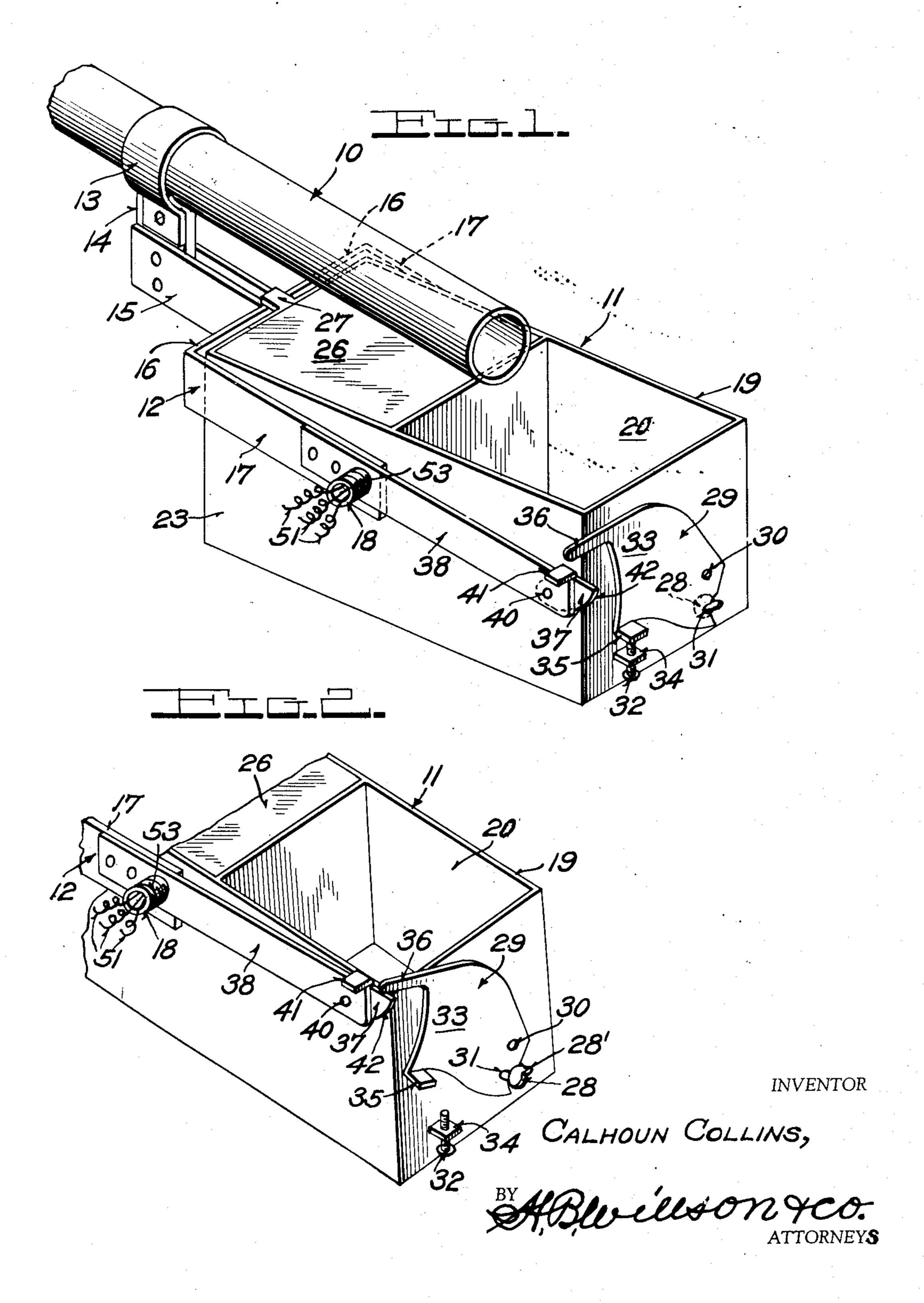
LIQUID CONTROLLED DEVICE WITH SELF-CLEANING VALVE
