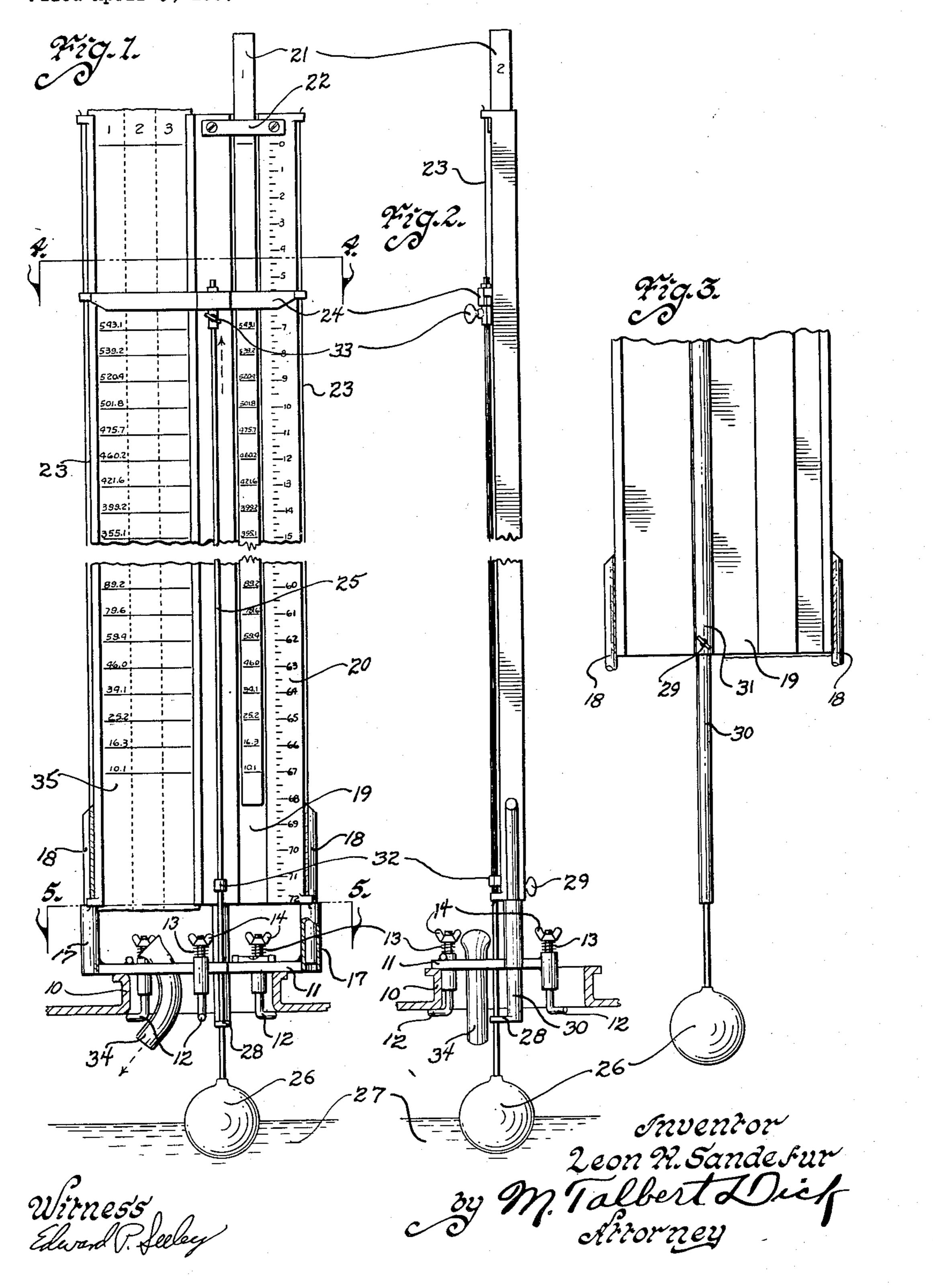
MEANS FOR CALIBRATING LIQUID LEVEL MEASURING STICKS
