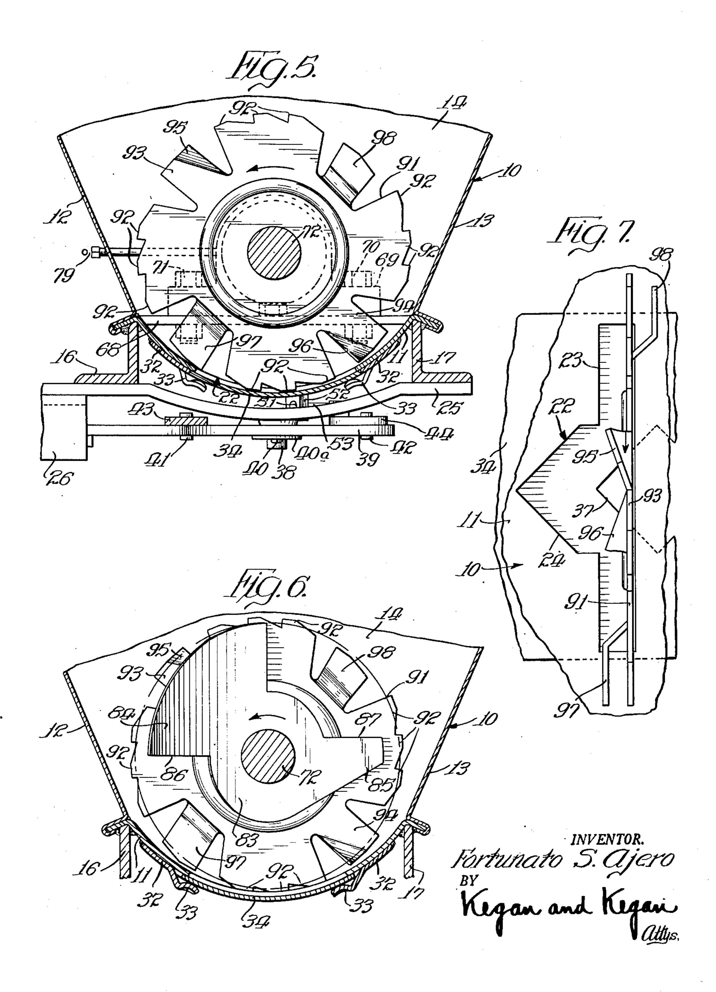
FEEDING MECHANISM FOR SPREADER AND SEEDER APPARATUS
