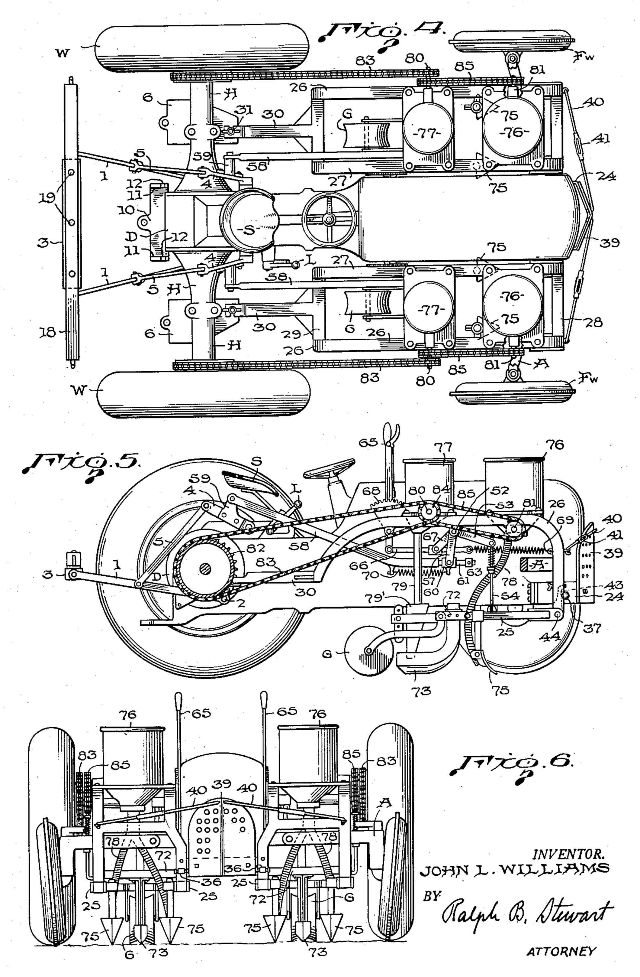
RIGID IMPLEMENT FRAME FOR FOUR-WHEELED TRACTORS
