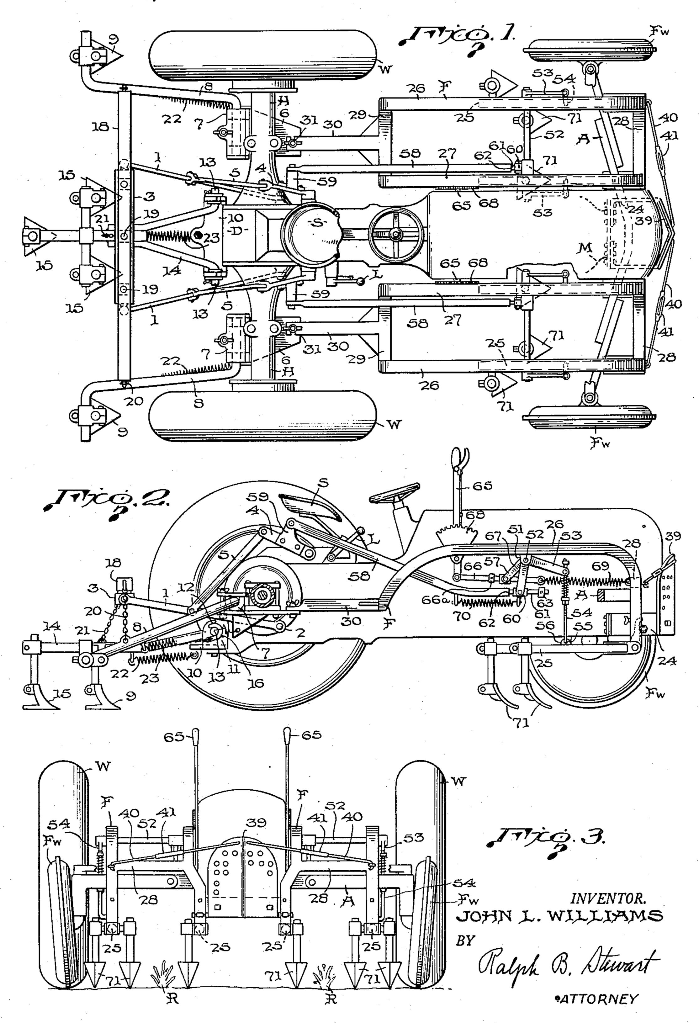
RIGID IMPLEMENT FRAME FOR FOUR-WHEELED TRACTORS
