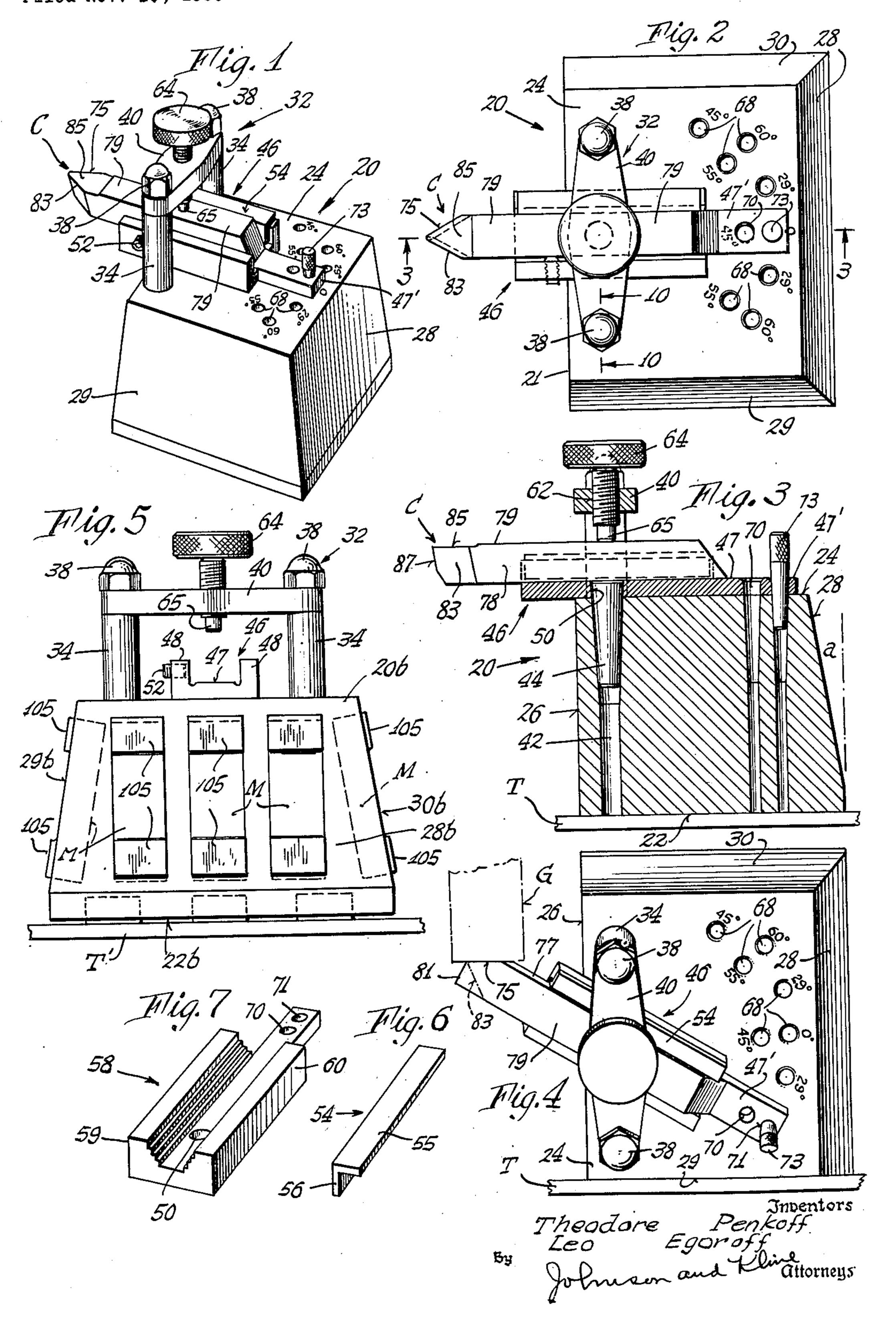
FIXTURE FOR GRINDING THREAD CUTTING TOOLS AND THE LIKE
