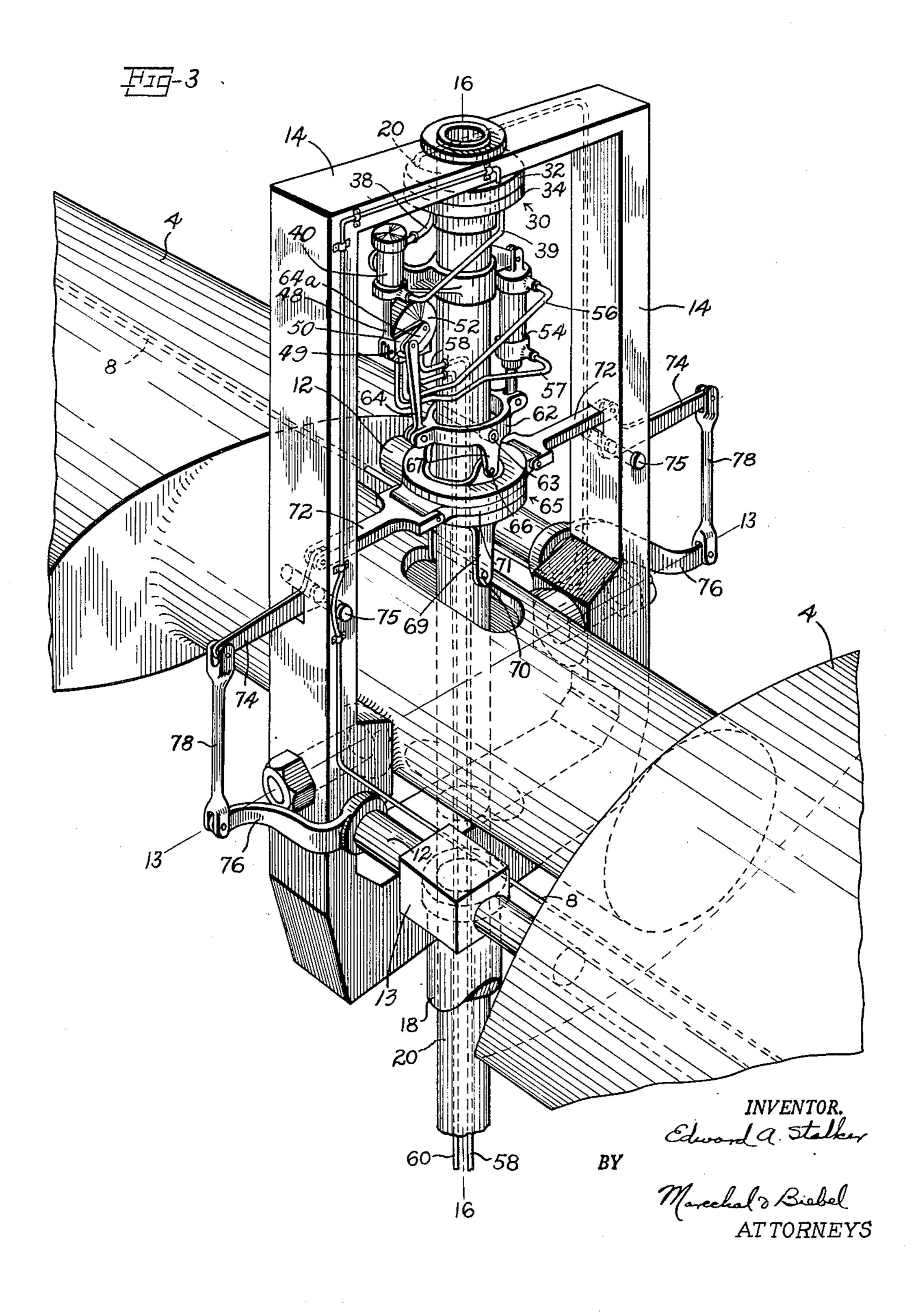
STABILIZING MECHANISM FOR ROTARY WING AIRCRAFT
