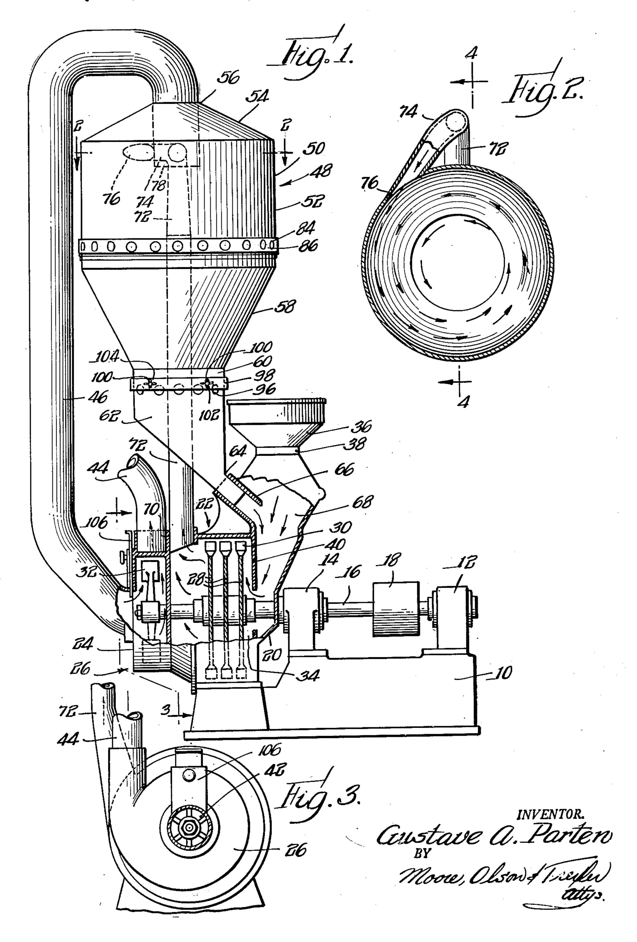
GAS SEPARATOR FOR GRINDING MILLS
