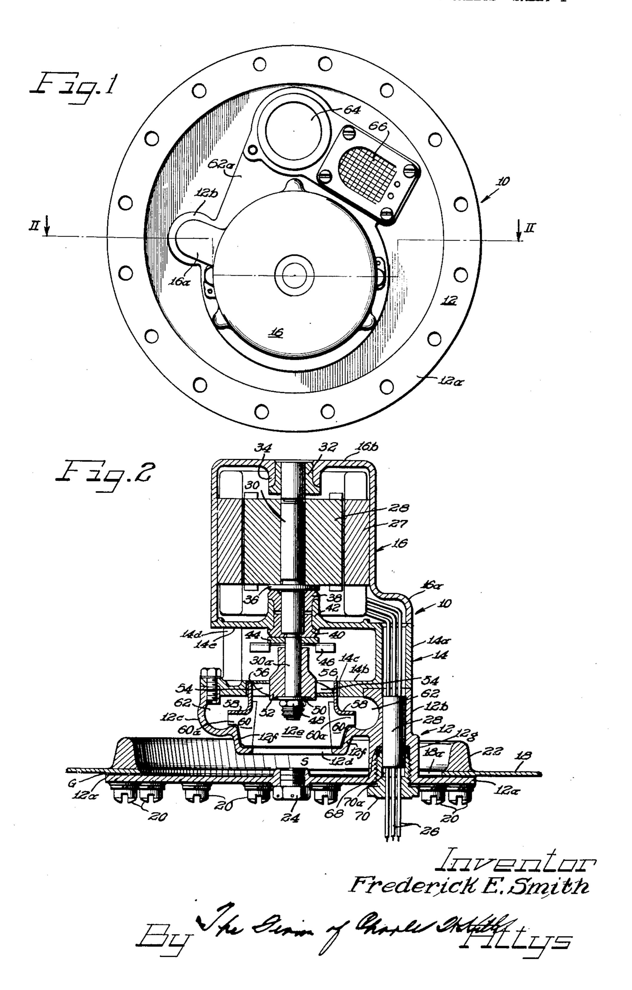
SUBMERGED PUMP AND MOTOR ASSEMBLY
