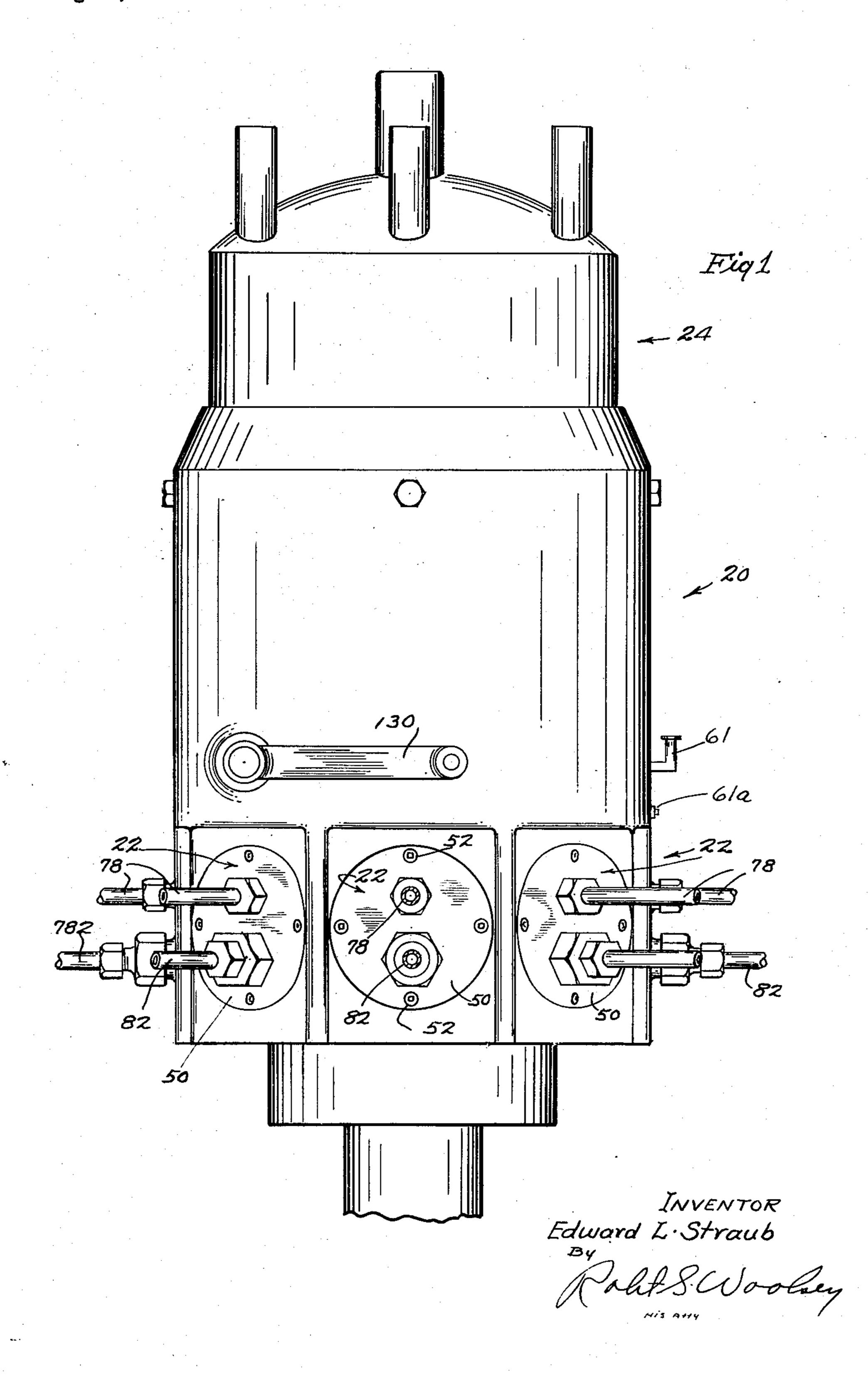
FUEL INJECTOR FOR INTERNAL-COMBUSTION ENGINES
