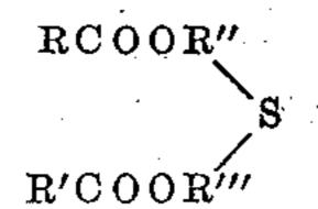
where R and R' each represent an alkyl radical containing 8 to 20 carbon atoms, at least one of such radicals having a branched chain, and where R'' and R''' each represent an alkylene radical containing 2 to 5 carbon atoms or a series of alkylene radicals interconnected by oxygen atoms, the number of carbon atoms in each such alkylene radical being 2 to 4 and the number of interconnected oxygen atoms being not greater
