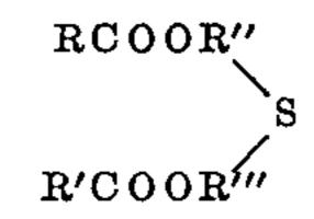
where R and R' are alkyl radicals containing 8 and 20 carbon atoms each, at least one of such 40 radicals being a C<sub>8</sub> to C<sub>11</sub> "Oxo" radical, and where R'' and R''' are alkylene radicals containing 2 to 5 carbon atoms each.
