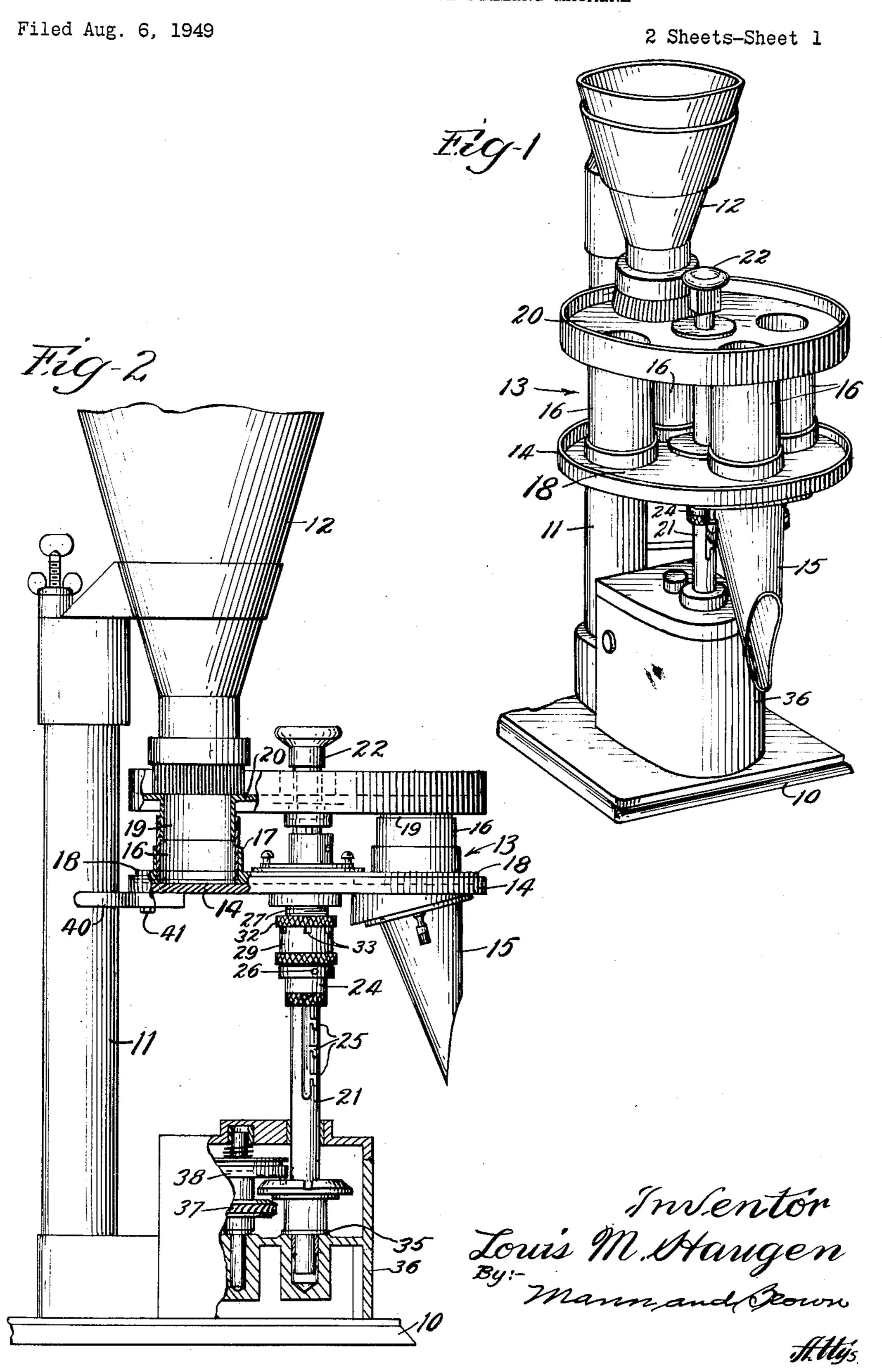
VOLUMETRIC PACKAGE FILLING MACHINE
