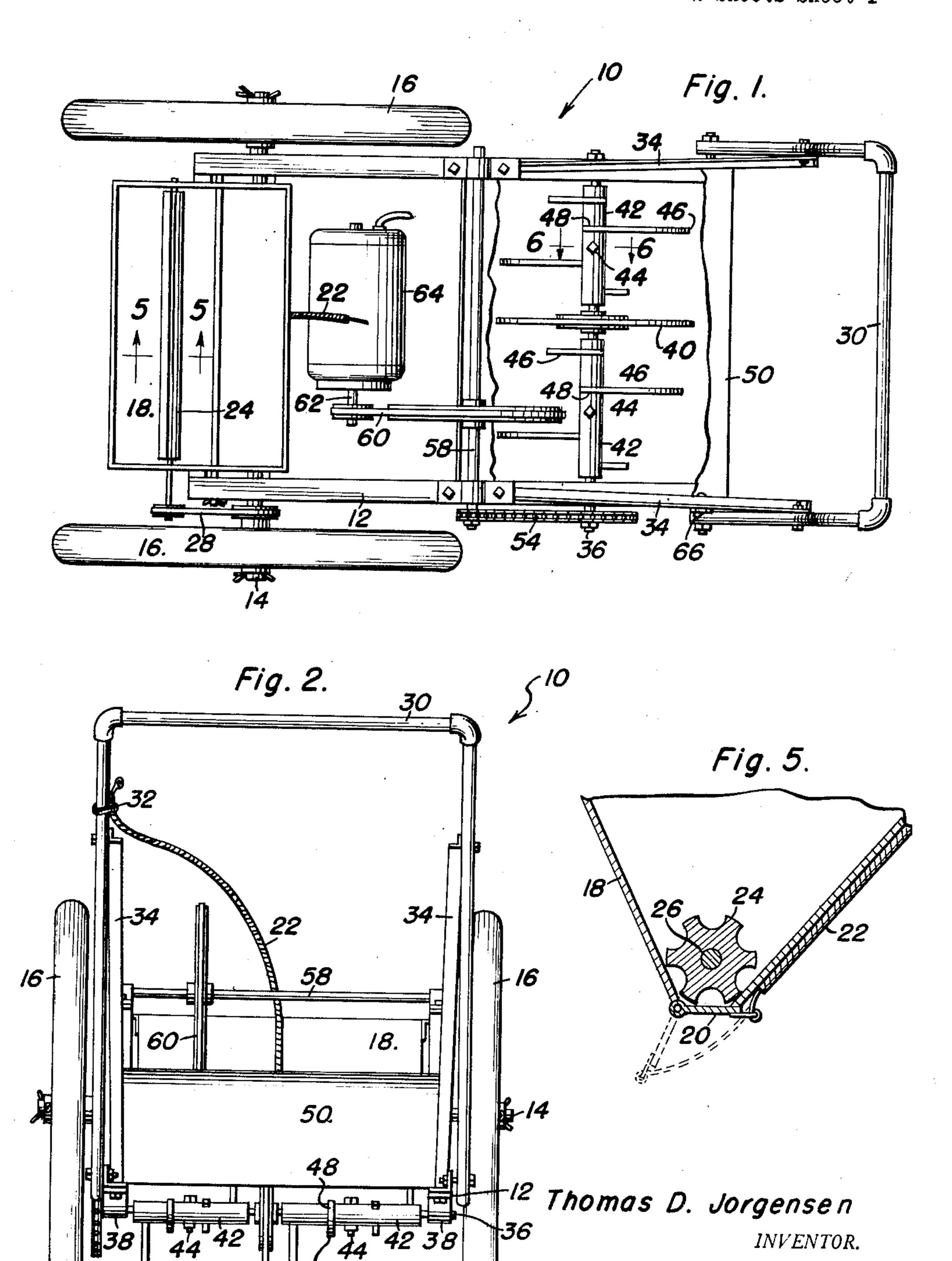
LITTER STIRRING AND LIME ADMIXING APPARATUS
