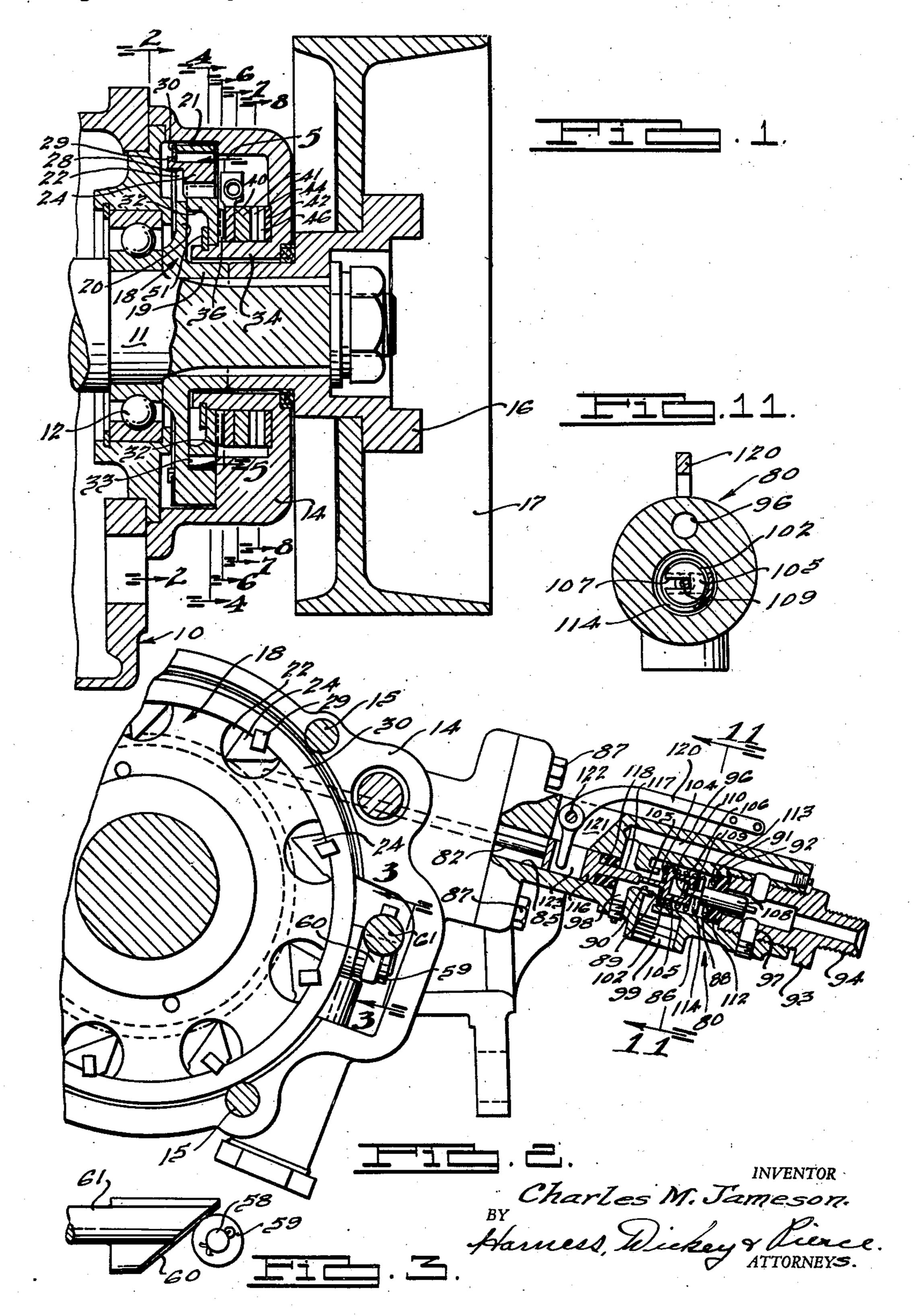
HOLDING VALVE DEVICE FOR FLUID OPERATED BRAKES
