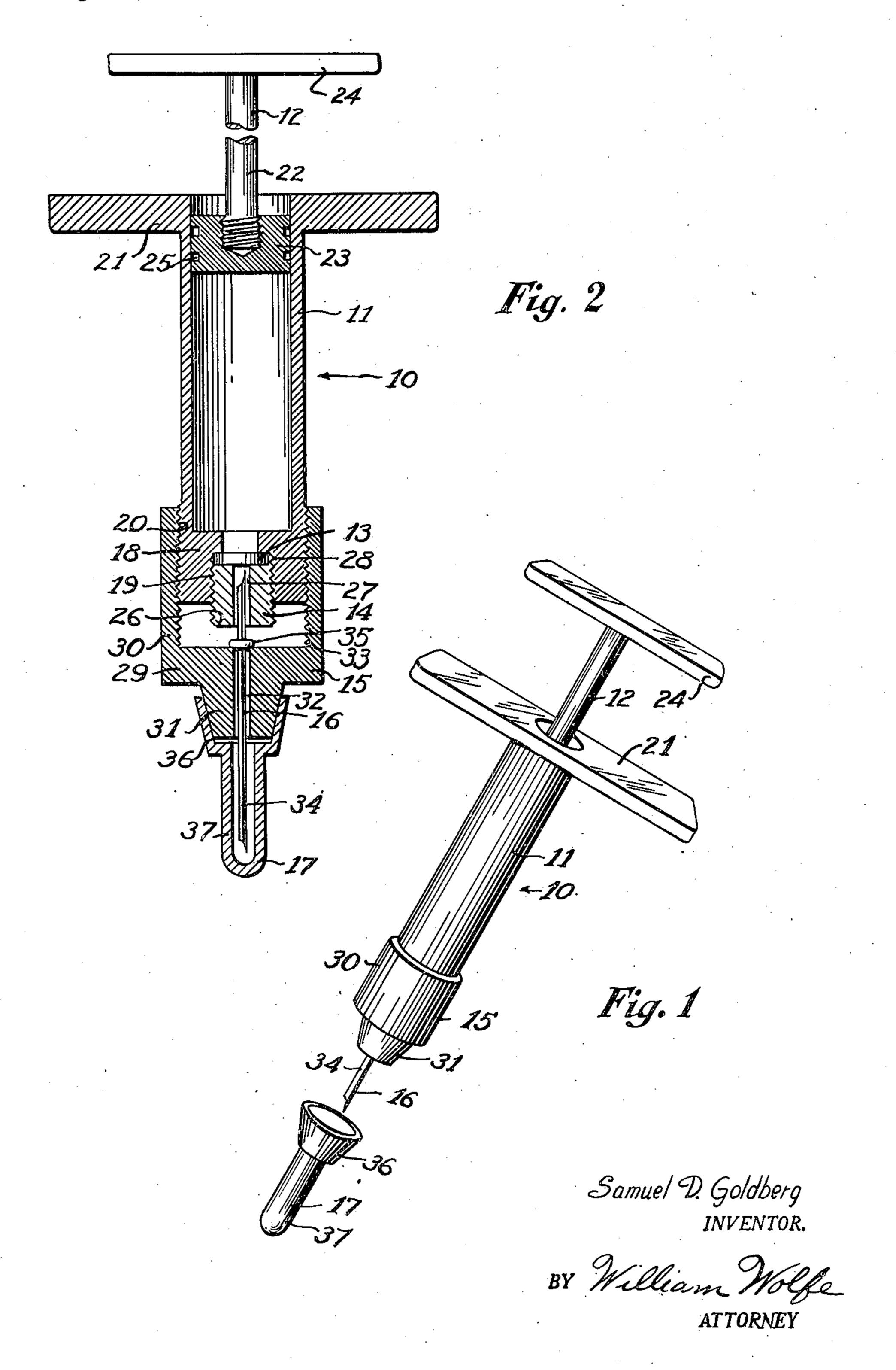
SYRINGE AND AMPOULE COMBINATION AND AMPOULE
