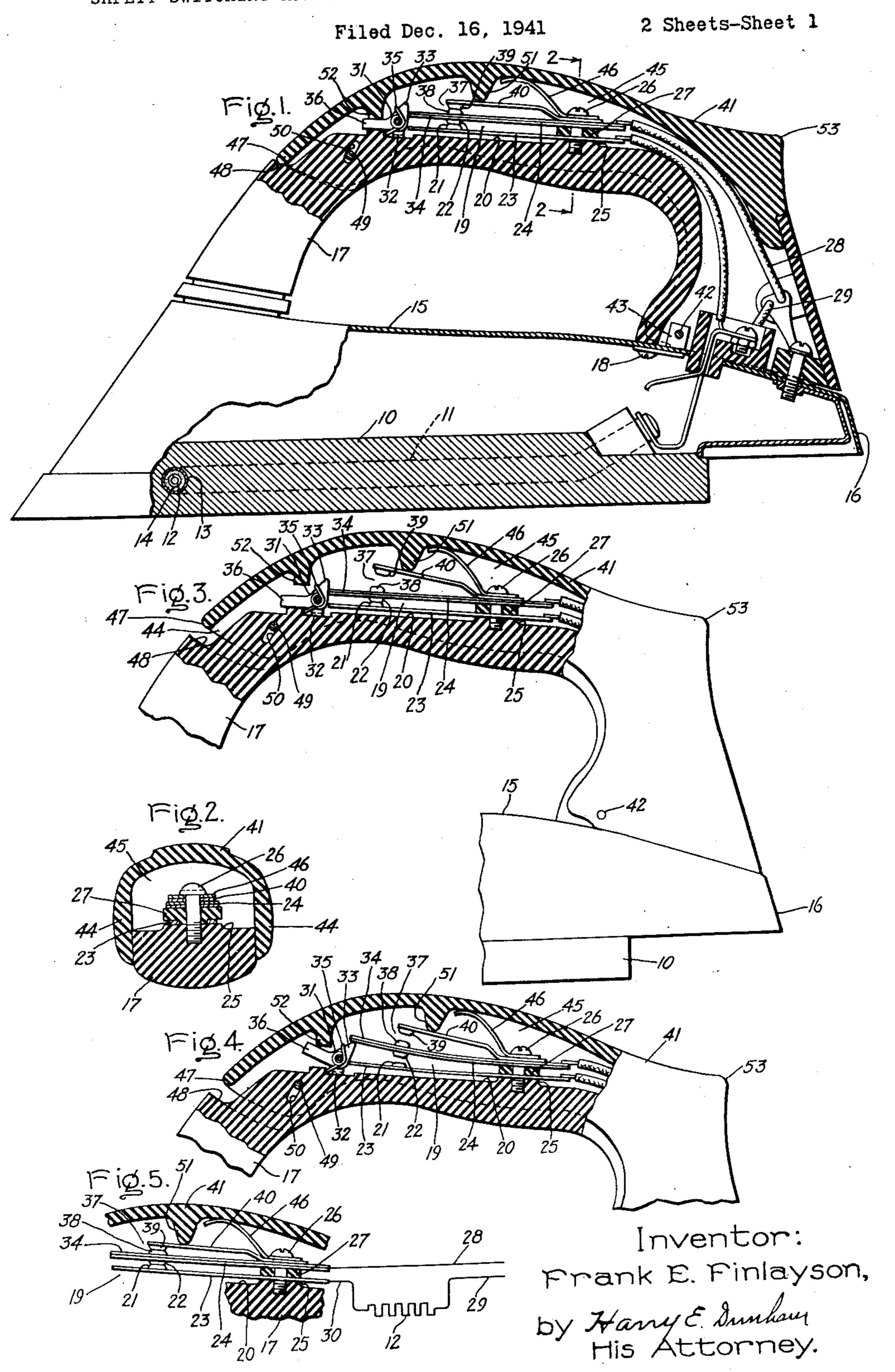
SAFETY SWITCHING ARRANGEMENT FOR ELECTRICALLY HEATED APPLIANCES
