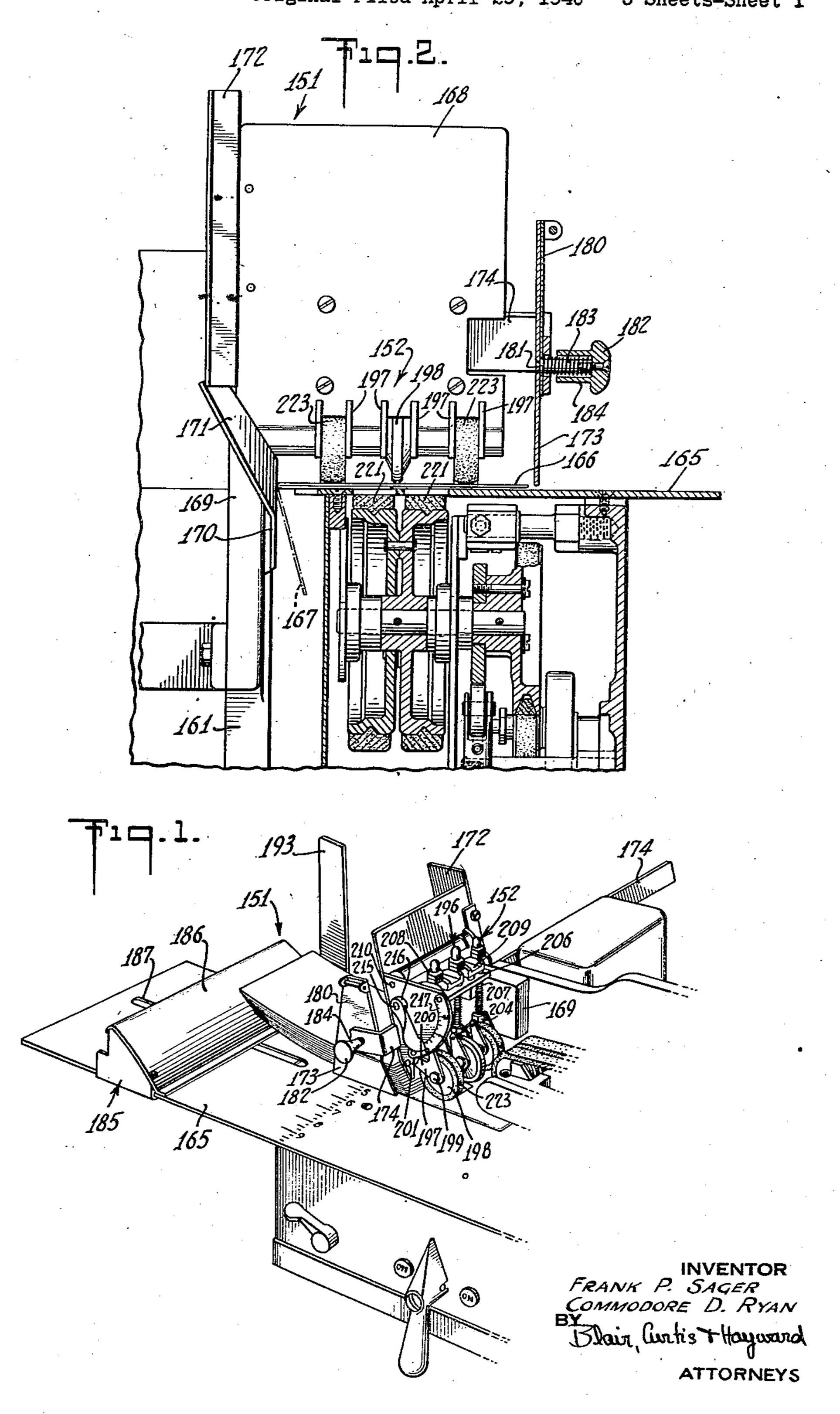
ENVELOPE HOPPER AND STRIPPING MECHANISM FOR MAIL TREATING APPARATUS
