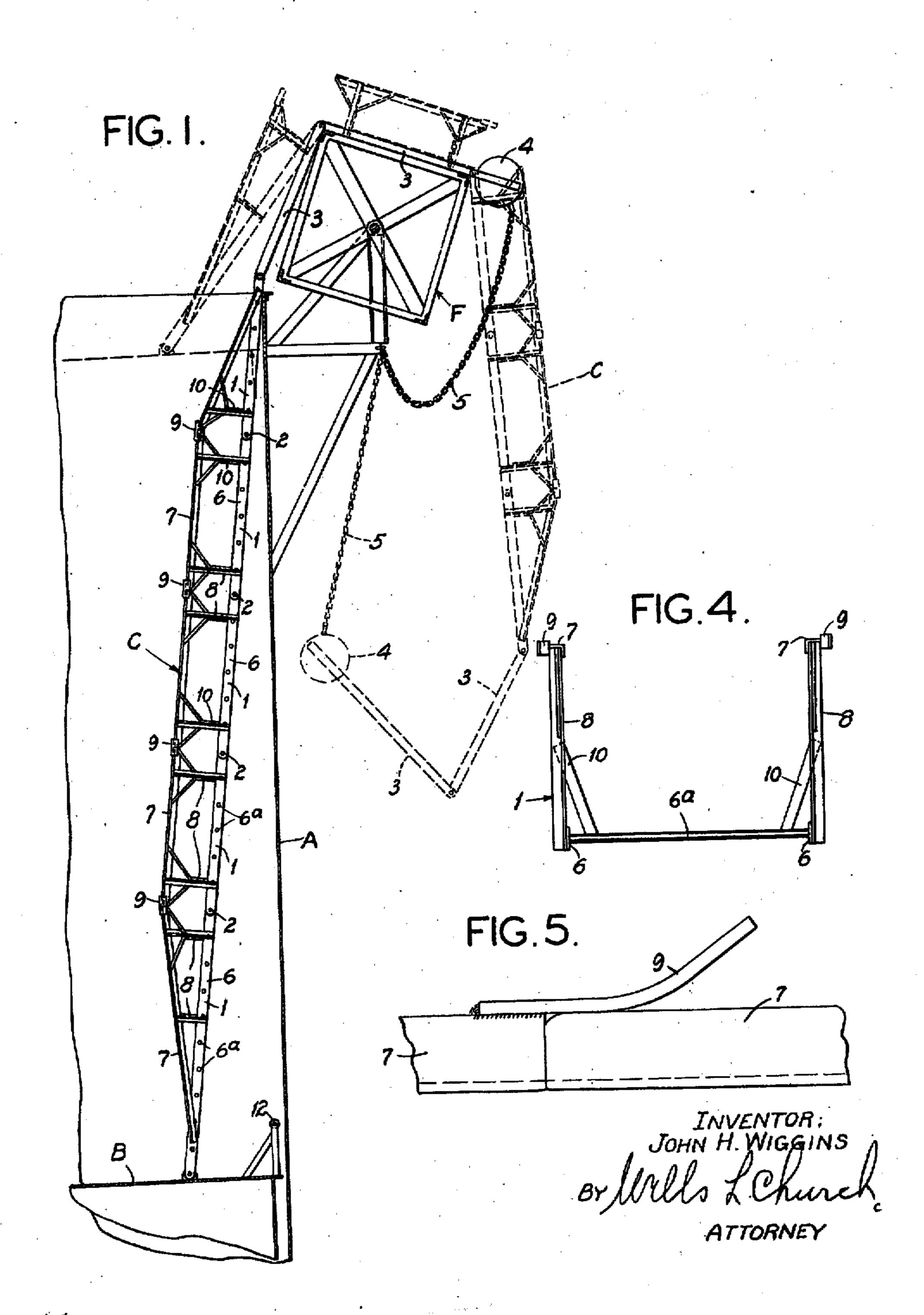
FOLDING LADDER AND SHIFTABLE PLATFORM FOR FLOATING TYPE TANK ROOFS
