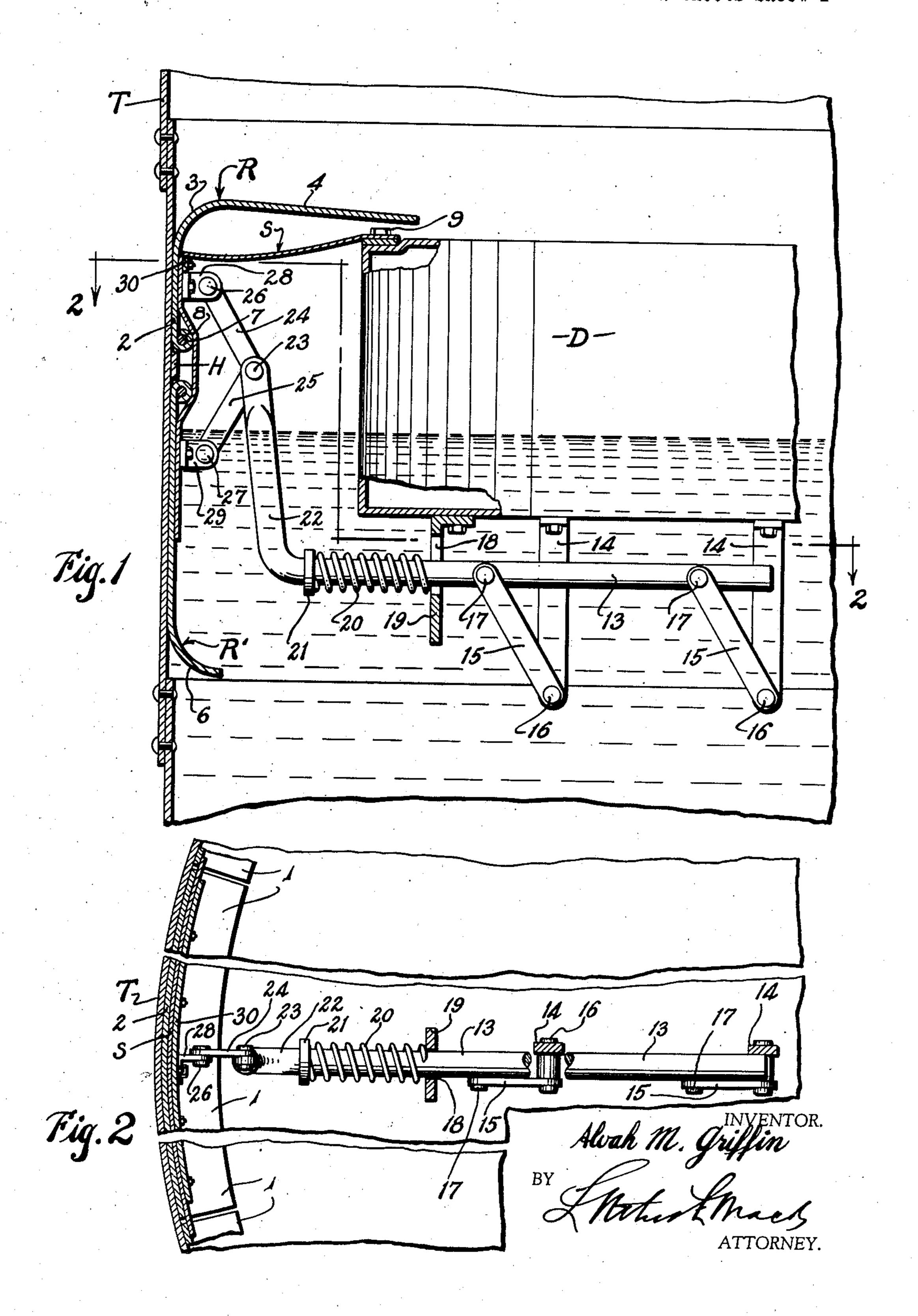
FLOATING DECK STRUCTURE FOR OIL STORAGE TANKS
