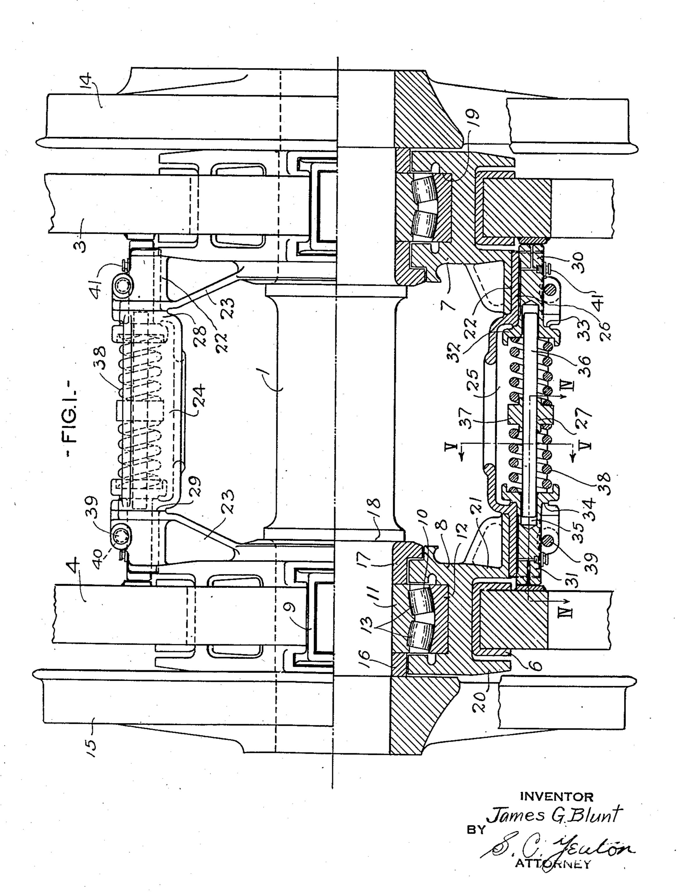
RAILWAY VEHICLE AND LATERAL MOTION RESISTANCE AND CENTERING DEVICE THEREFOR
