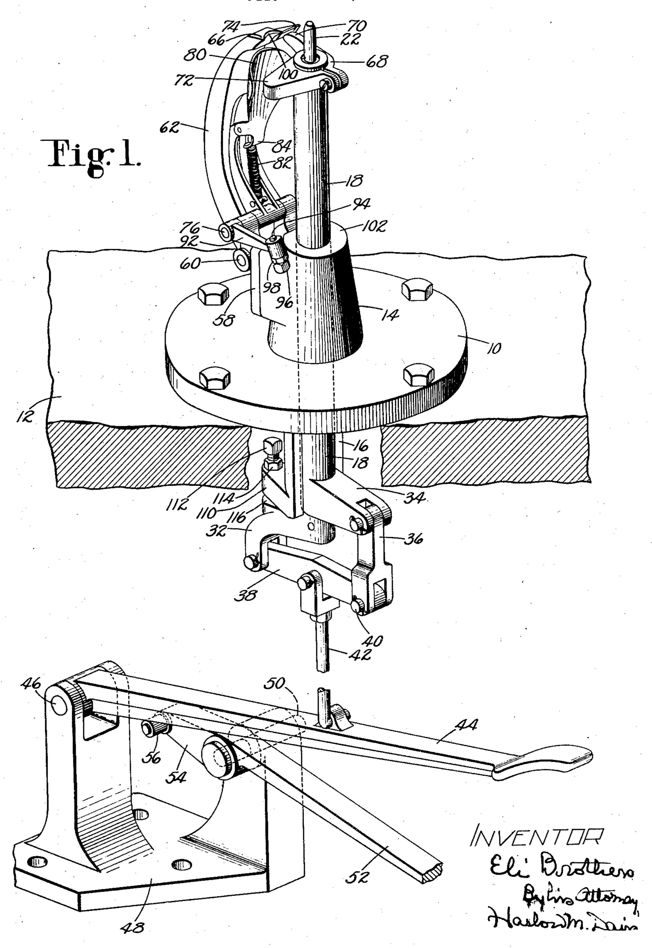
MACHINE FOR EFFECTING RELATIVE MOVEMENT BETWEEN LASTS AND SHOES
