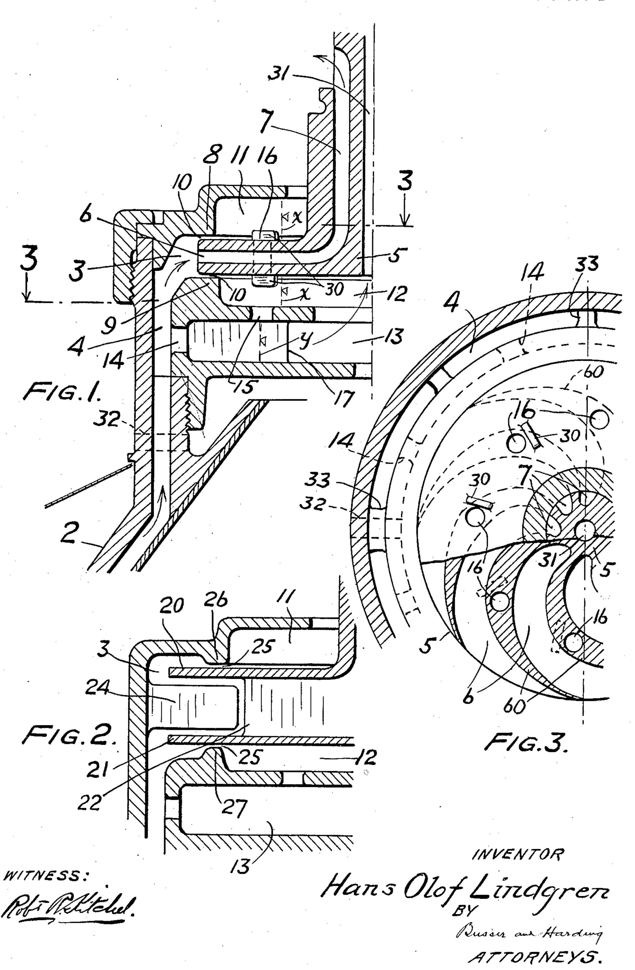
ANTIFROTH DISCHARGING MEANS FOR CENTRIFUGAL SEPARATORS
