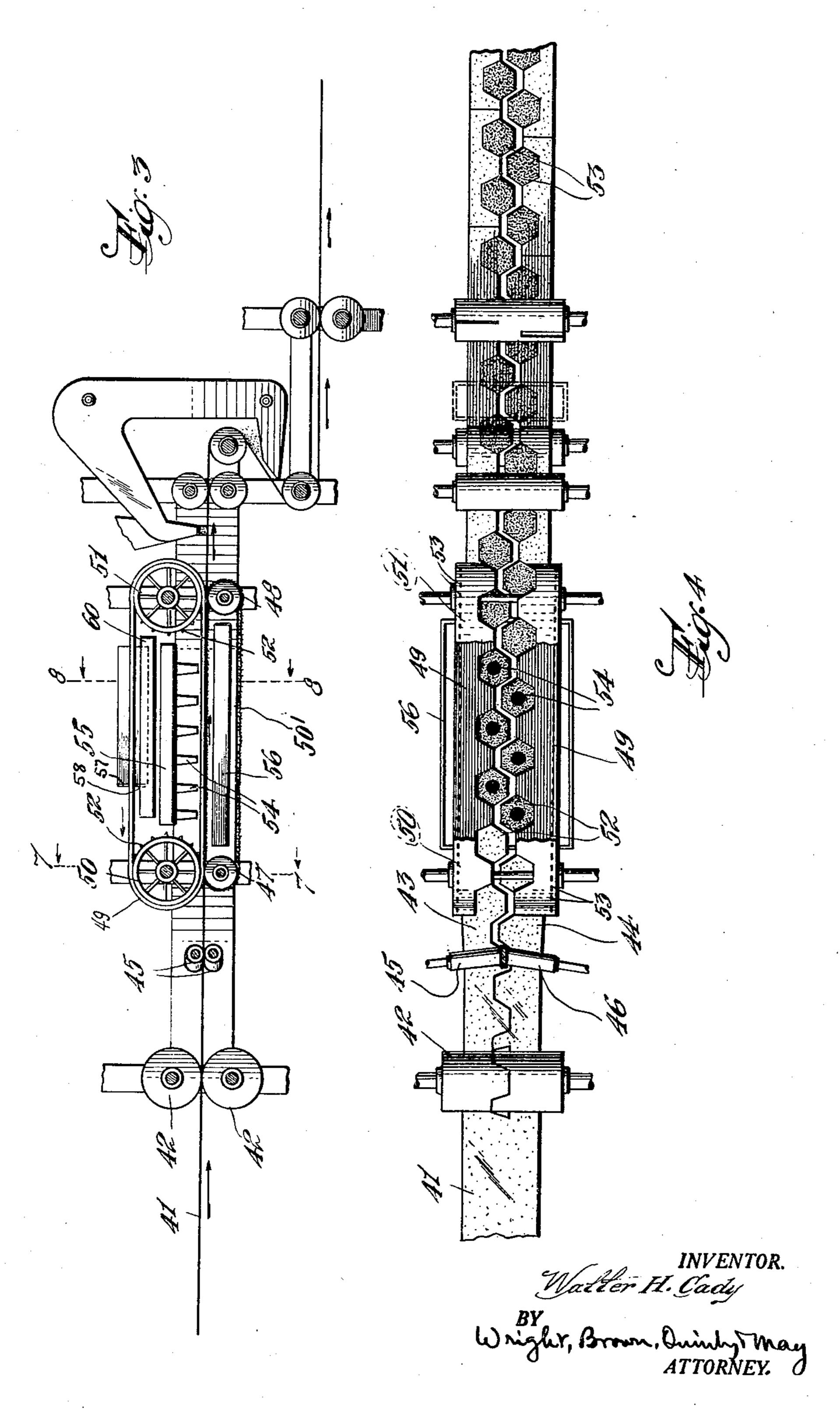
METHOD AND APPARATUS FOR TREATING SHINGLES OR SHINGLE STRIPS
