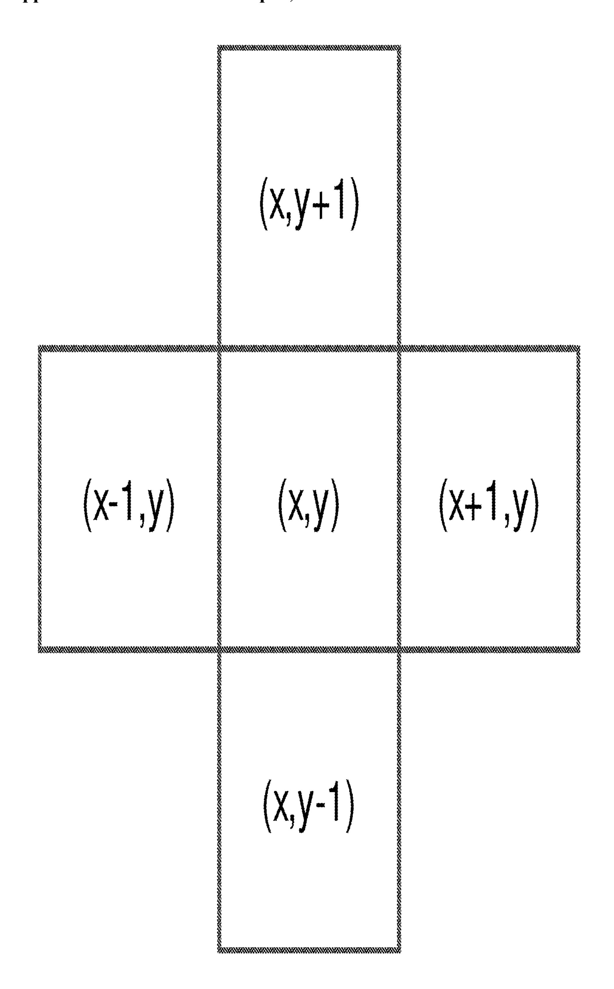
Figure 1: Star-Shaped Convolution Filter, "star-conv"
