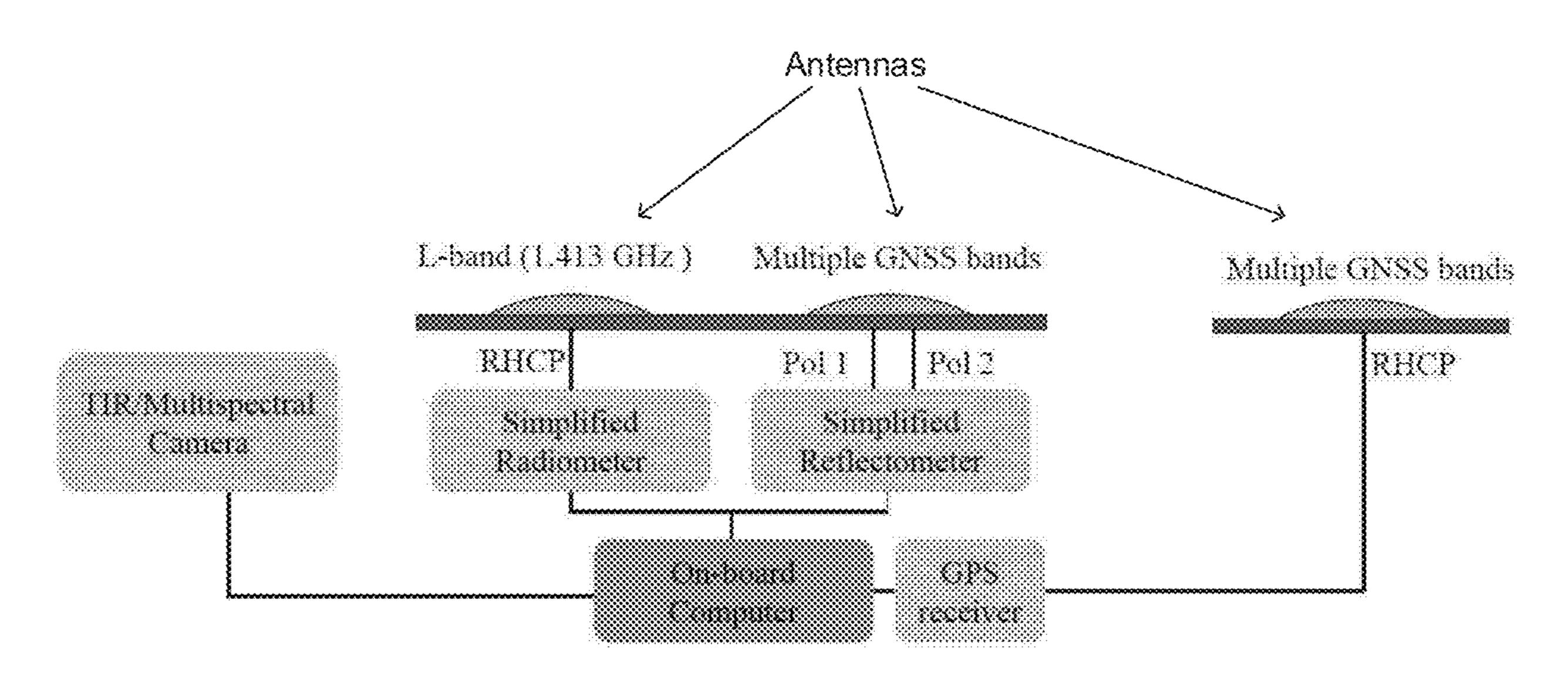
Pol 1/Pol 2 can be any combination of orthogonal polarizations: RHCP LHCP or H/V.
