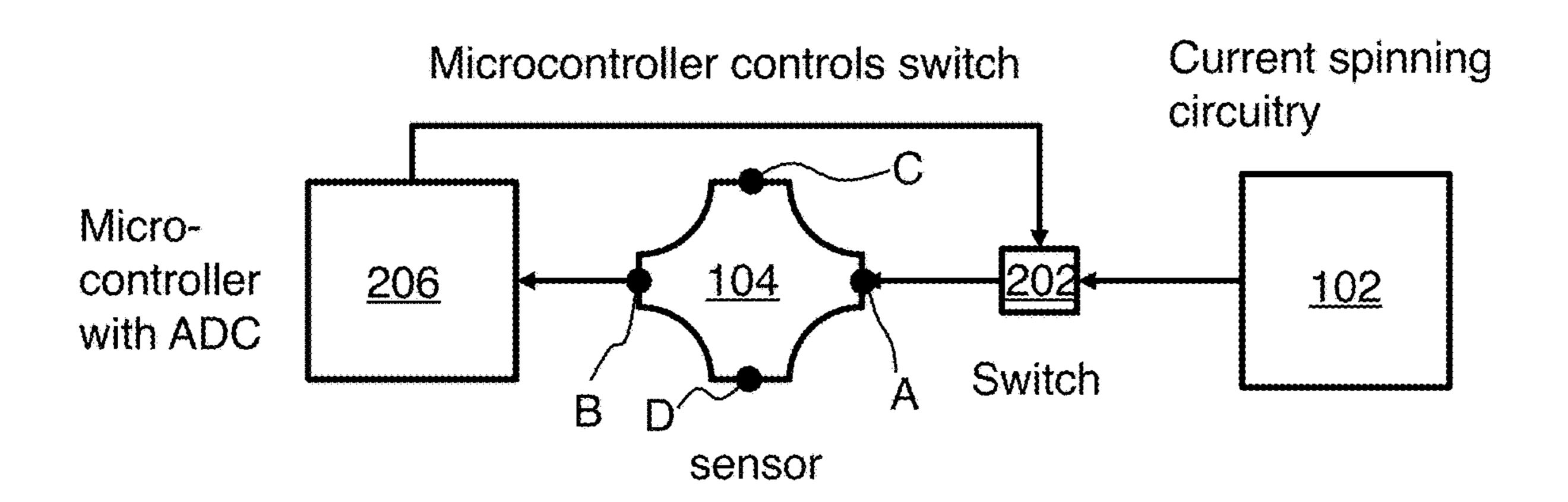
switch 202 closed => Hall effect measurement with current spinning switch 202 open => inductive measurement, no current in sensor
