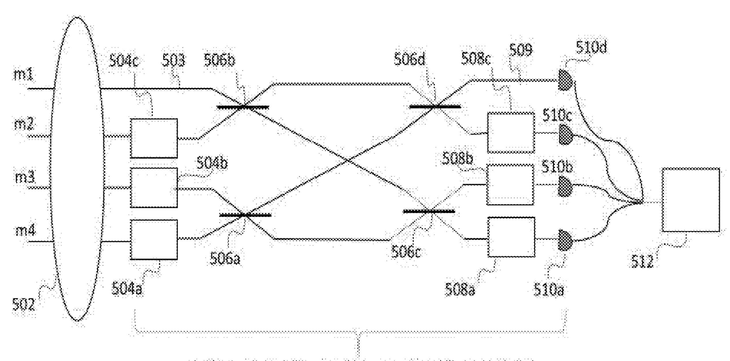
Optical domain processing to perform the Quantum Fourier Transform
