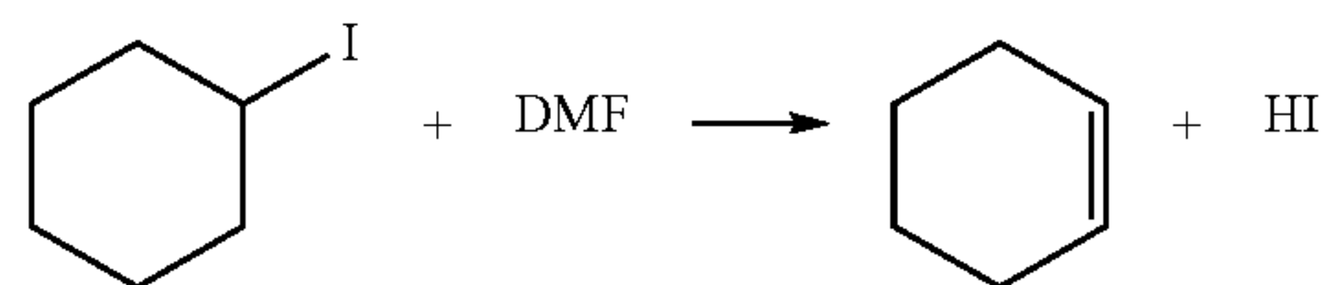
Scheme 6: Reaction of iodocyclohexane in situ for deprotection of poly(catechol-styrene).
