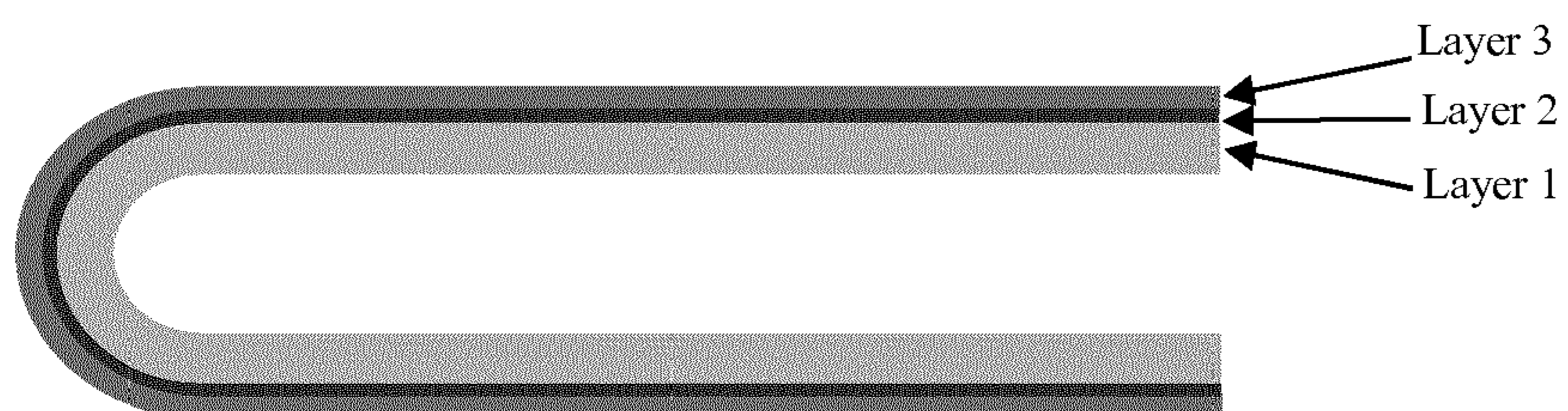
Figure 5: Tubular design illustrating the support (layer 1), the membrane (layer 2) and the electrode (layer 3).
