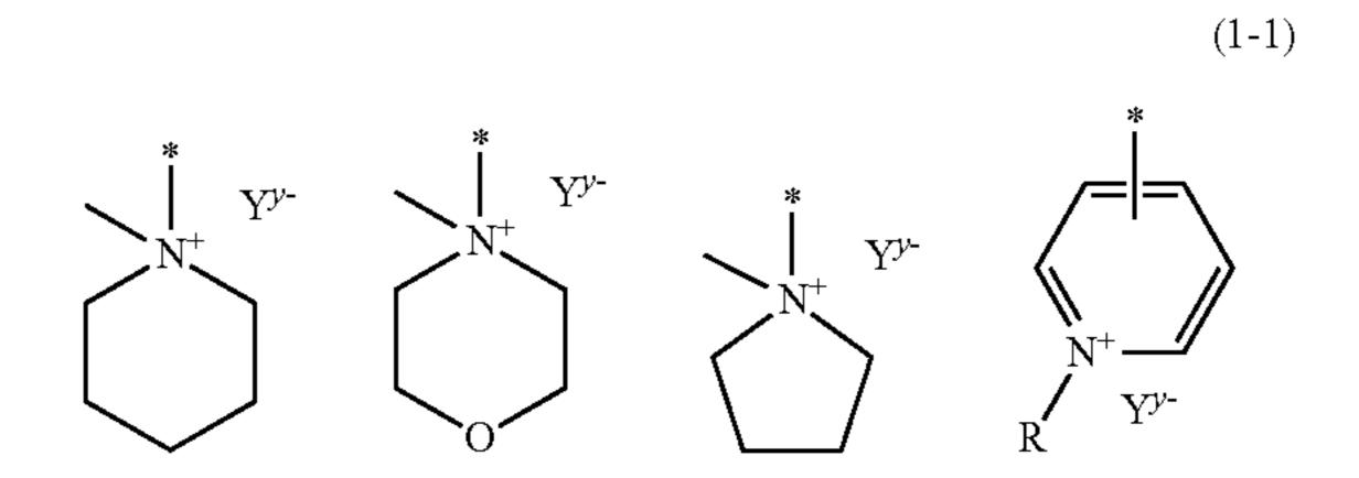
[0053] In formula (1-1) R represents a hydrogen atom, or a substituted or unsubstituted hydrocarbon group,  $Y^{y-}$  represents a y-valent counter anion, and "\*" represents a chemical bond. As the hydrocarbon group for R, one similar to that described above for  $R^2$  can be mentioned, and as the  $Y^{y-}$ , one similar to  $Y^{y-}$  in the above-described — $N^+R^2R^3R^4Y^{y-}$  can be mentioned.
