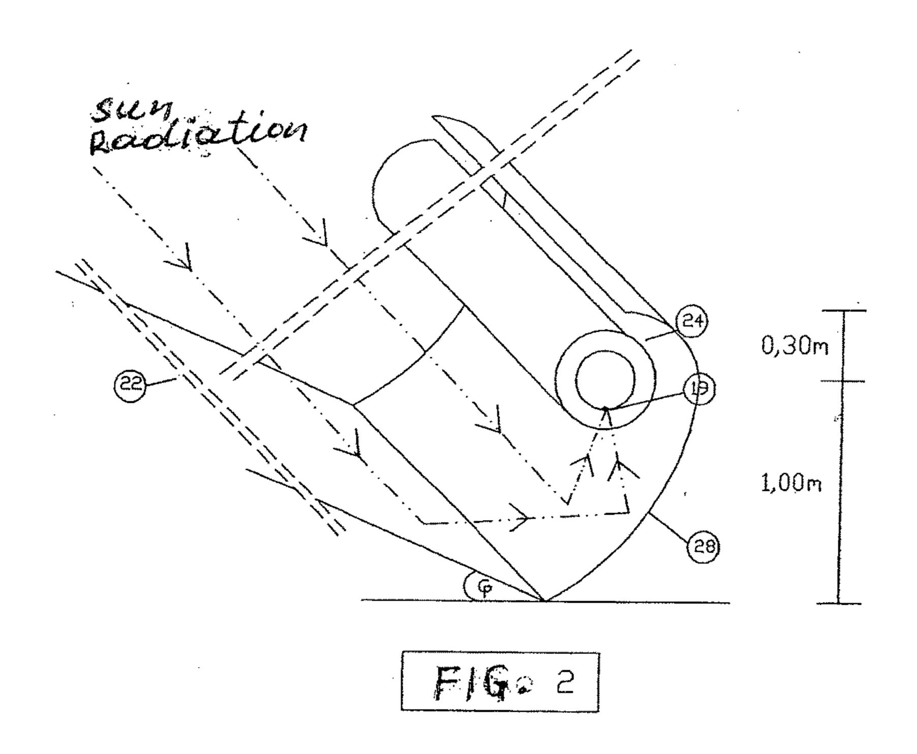
SOLAR COLLECTOR OF PHOTOVOLTAIC SYSTEM, IN TUBE FORM, WITH ARRAYS OF CONCENTRATING CELLS, WATER COOLED, IN THE FOCUS OF SEMI CYLINDRICAL, STABLE, PARABOLIC REFLECTOR FOR THE PRODUCTION OF ELECTRICAL AND THERMAL ENERGY
