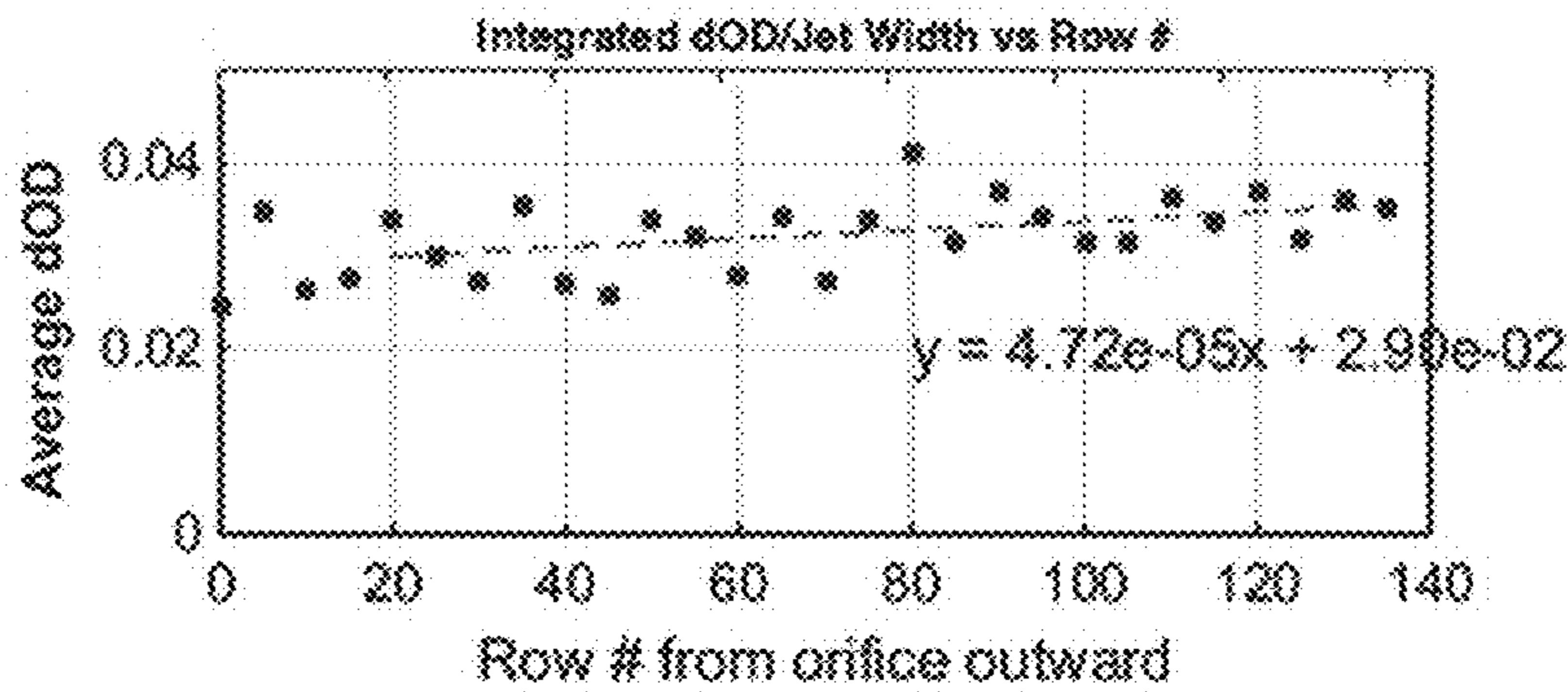
Integrated Optical Depth Across Jet from a 50um Slit
