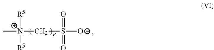
wherein  $R^1$  is independently at each occurrence a substituted or unsubstituted  $C_{1-12}$  alkyl group; and  $p$  is independently at each occurrence an integer from 1 to 12. In some embodiments, each occurrence of  $R^5$  is methyl. In some embodiments,  $p$  is an integer from 1 to 6, for example, in some embodiments  $p$  is equal to 3.
