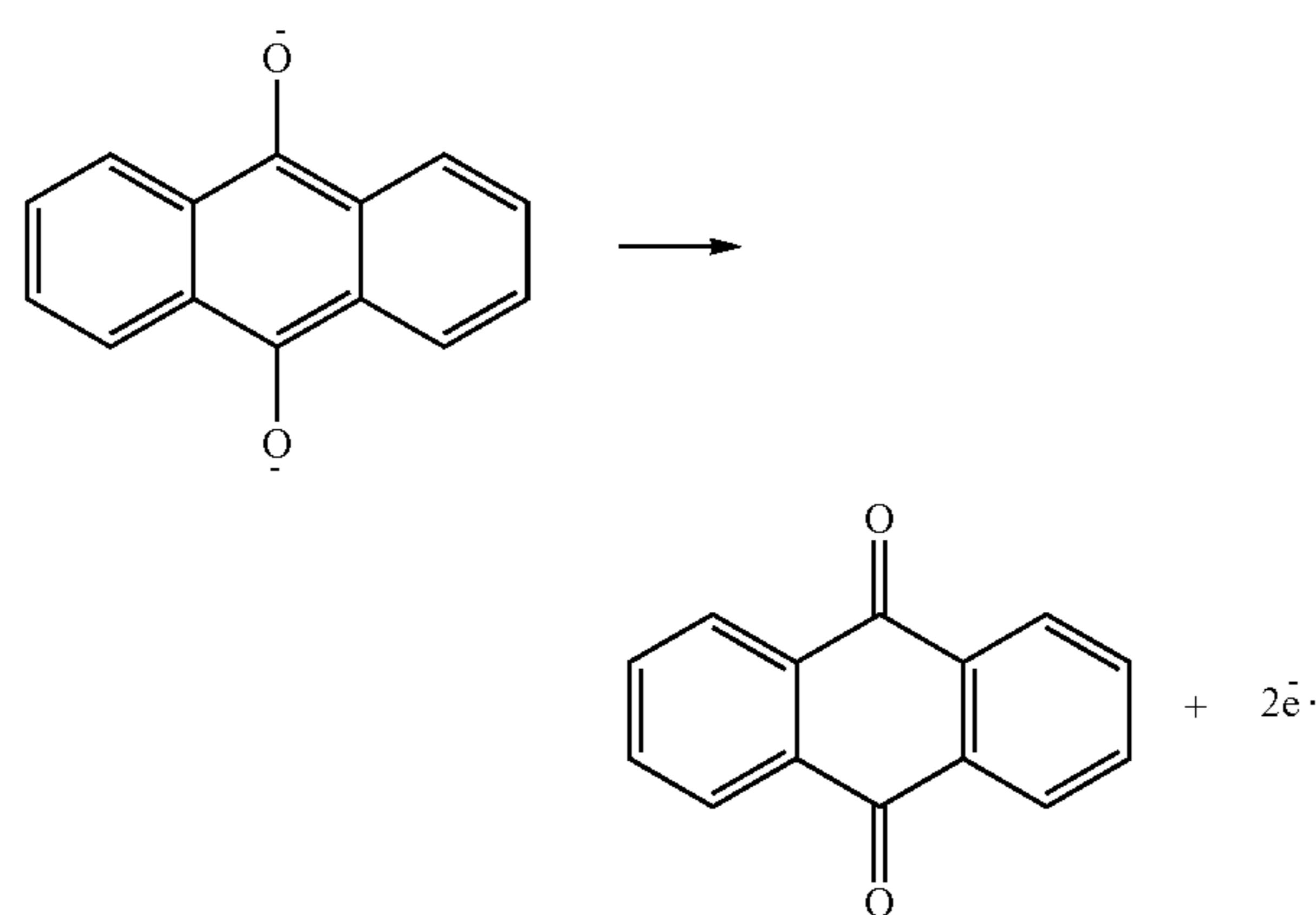
[0061] According to some embodiments in which the electroactive active species is oxidized after bonding to a target species comprising carbon dioxide, the following reaction (5) may take place:
