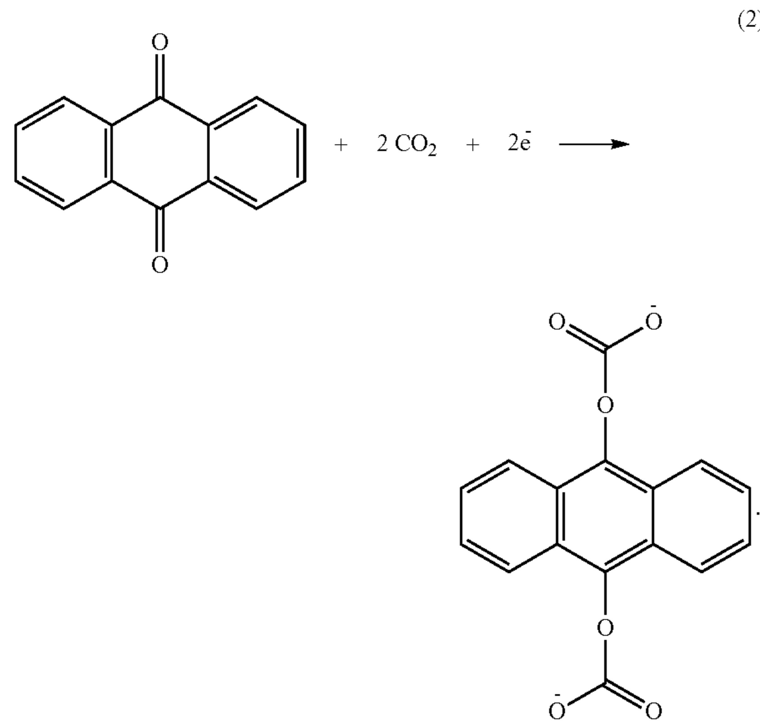
[0052] According to some embodiments, while the first electroactive species (e.g., polyanthraquinone) is being reduced at the negative electrode, the second electroactive species (e.g., polyvinyl ferrocene) is being oxidized at the positive electrode. During the charge mode, the oxidation of the second electroactive species provides a source of electrons for driving the reduction of the first electroactive species.
