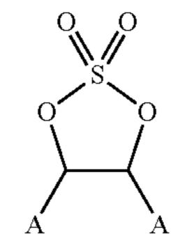
wherein each A is independently a hydrogen or an optionally fluorinated vinyl, allyl, acetylenic, propargyl, or C<sub>1</sub>-C<sub>3</sub> alkyl group. The electrolyte compositions are useful in electrochemical cells, such as lithium ion batteries.
