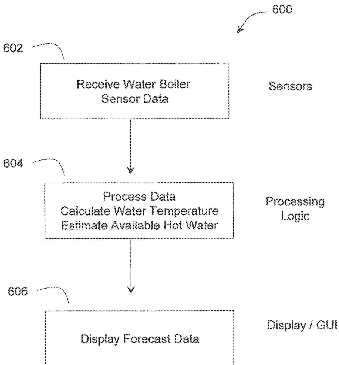
**FIG. 7** RECEIVING SENSOR DATA SUBROUTINE
